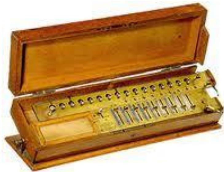
**Gambar 7.5** Kalkulator Roda Mekanik
