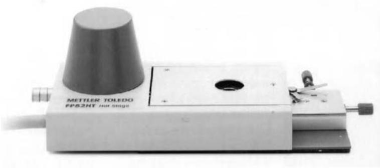
**FIGURE 7.6** Mettler FP84HT hot-stage accessory. (From Rapid and Automatic Determination of Thermal Values Product Brochure, Mettler-Toledo Company, Hightstown, NJ, 1996. With permission.)
