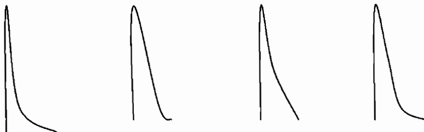
Figure 45-1. Typical tailing peak shapes in HPLC.
