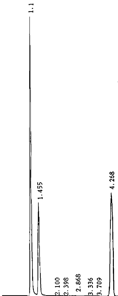
Figure 4-1. "Separation" of pyridine/benzylamine, uracil (inert!), phenol in an acidic phosphate buffer with a hydrophobic RP phase.
