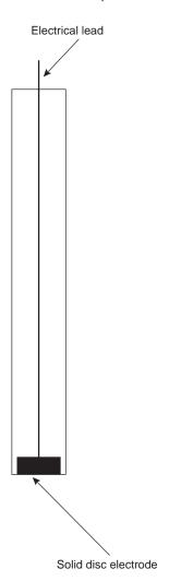
**Figure 11.27** Schematic diagram of a solid electrode.
