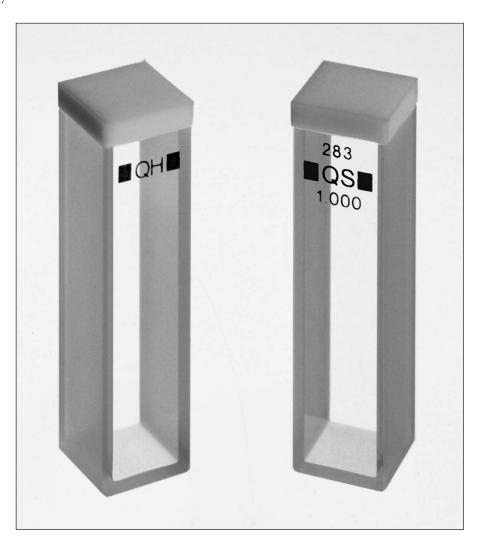
**Figure 10.29**Typical cells used in UV/Vis spectroscopy.
