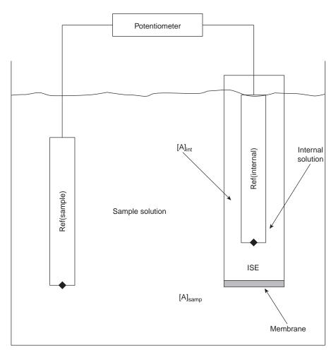
Figure II.10 Electrochemical cell for potentiometry with an ion-selective membrane electrode.
