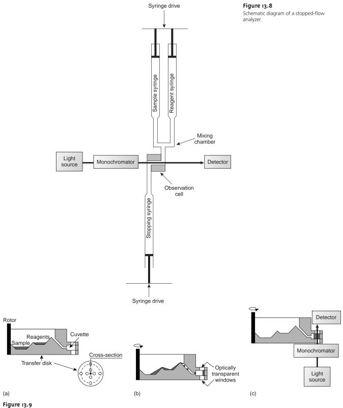
Schematic diagram of a centrifugal analyzer showing (a) the wells for holding the sample and reagent; (b) mixing of the sample and reagent; and (c) the configuration of the spectrophotometric detector.
