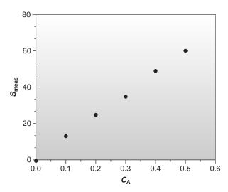
**Figure 5.8**Normal calibration plot of hypothetical data from Table 5.1.
