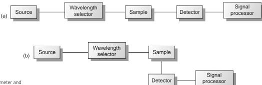
**Figure 10.54**Block diagrams for (a) a turbidometer and (b) a nephelometer.
