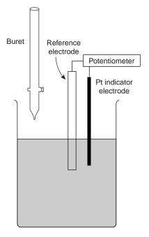
**Figure 9.38**Experimental arrangement for recording a potentiometric redox titration curve.
