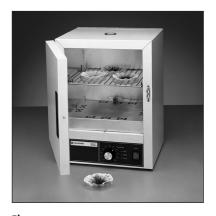
**Figure 2.7**Conventional laboratory oven used for drying materials.
