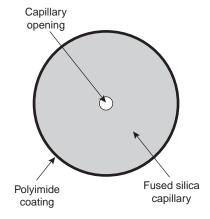
**Figure 12.42**Schematic diagram showing a cross section of a capillary column for capillary electrophoresis.
