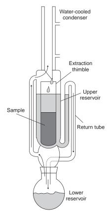
**Figure 7.18**Schematic diagram of a Soxhlet extractor.
