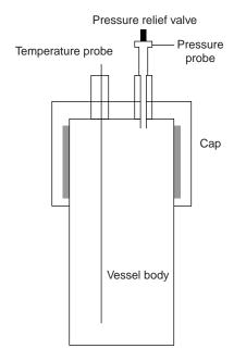
**Figure 7.10**Schematic diagram of a microwave digestion vessel
