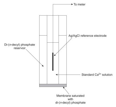
**Figure 11.14**Schematic diagram of a Ca<sup>2+</sup> liquid-based ion-selective electrode.
