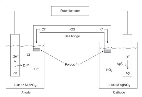
**Figure 11.5** Electrochemical cell for potentiometry.
