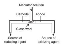
**Figure 11.25**Method for the external generation of oxidizing and reducing agents in coulometric
