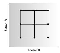
**Figure 14.14**  $3^k$  factorial design for k = 2.
