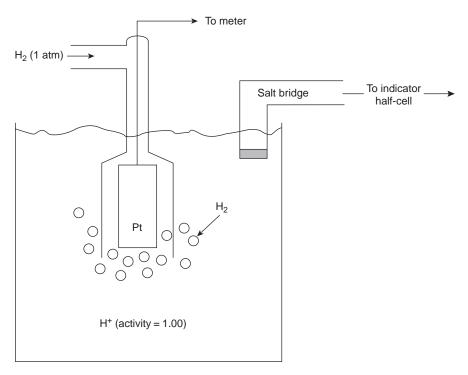
**Figure 11.7**Schematic diagram of the standard hydrogen electrode (SHE).
