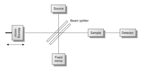
**Figure 10.13**Block diagram of an interferometer.
