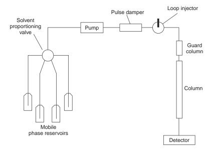
**Figure 12.26**Schematic diagram of a high-performance liquid chromatograph.
