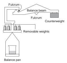
**Figure 2.3**Schematic diagram of single-arm mechanical balance.
