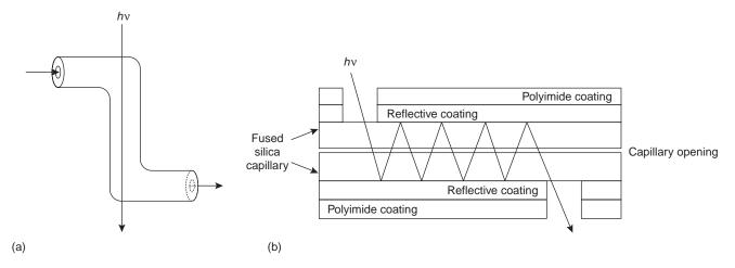
Figure 12.44 Schematic diagrams of two approaches to on-column detection using UV/Vis absorption spectroscopy.
