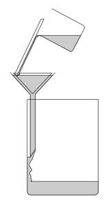
**Figure 8.7**Proper procedure for transferring the supernatant to the filter paper cone.
