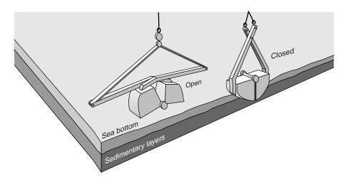
**Figure 7.5**Schematic diagram of grab sampler. When the sampler reaches the sediment, the jaws of the grab sampler are closed, collecting a sample of the sediment.
