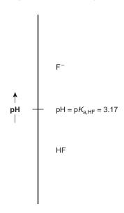
**Figure 6.4**Ladder diagram for HF, showing areas of predominance for HF and F<sup>-</sup>.
