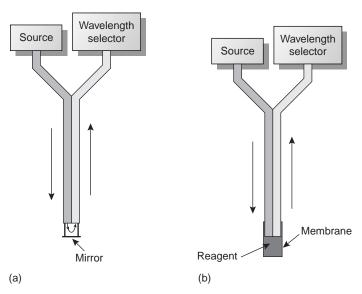
**Figure 10.30** Example of fiber-optic probes.
