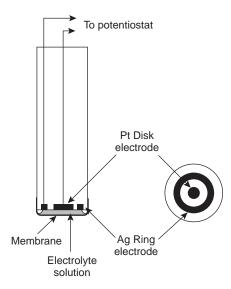
**Figure 11.38**Clark amperometric sensor for the determination of dissolved O<sub>2</sub>.
