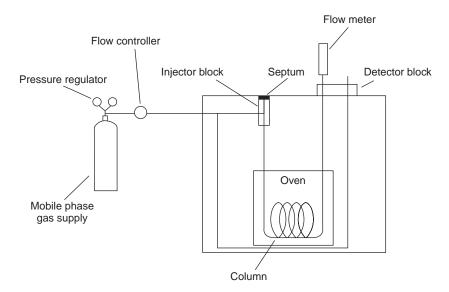
**Figure 12.16**Schematic diagram for a typical gas chromatograph.
