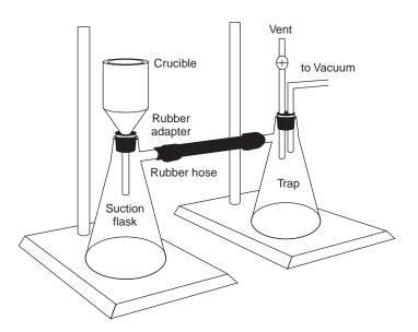
**Figure 8.8**Procedure for filtering through a filtering crucible. The trap is used to prevent water from a water aspirator from backwashing into the suction flask.
