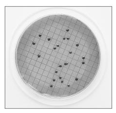
**Figure 3.1**Membrane filter showing colonies of coliform bacteria. The number of colonies are counted and reported as colonies/100 mL of sample.
