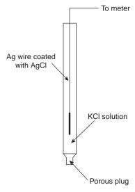
**Figure 11.9**Schematic diagram of a Ag/AgCl electrode.
