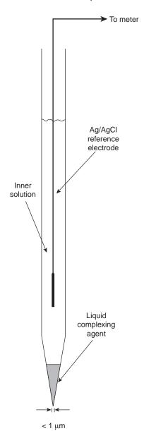
**Figure 11.19**Schematic diagram of a liquid-based ion-selective microelectrode.
