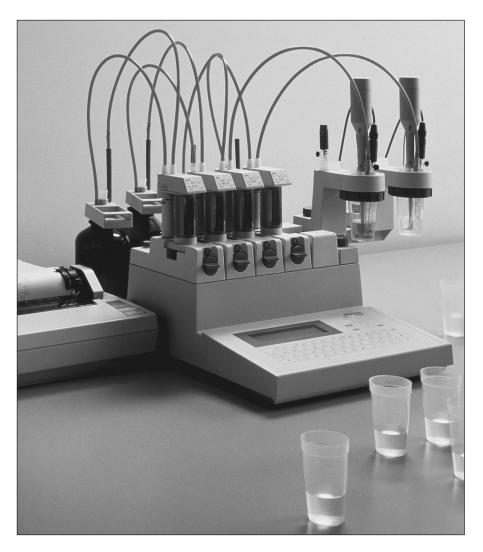
**Figure 9.5**Typical instrumentation for performing an automatic titration.
