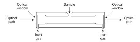
**Figure 10.40**Diagram of an electrothermal analyzer.
