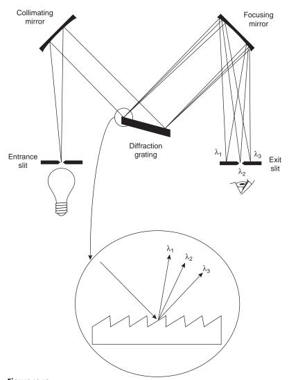
**Figure 10.12**Typical grating monochromator with inset showing the dispersion of the radiation by the diffraction grating.
