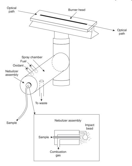
**Figure 10.38**Flame atomization assembly equipped with spray chamber and slot burner. The inset shows the nebulizer assembly.
