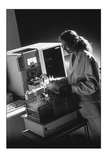
**Figure 10.37**Photo of a typical atomic absorption spectrophotometer.
