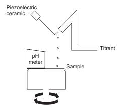
**Figure 9.22**Experimental design for a microdroplet titration apparatus.
