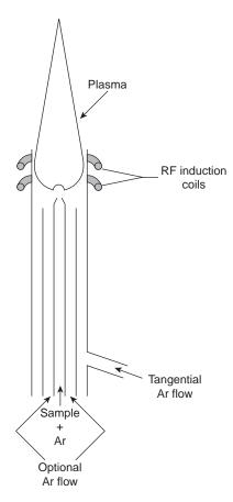
**Figure 10.49**Diagram of an inductively coupled plasma torch.
