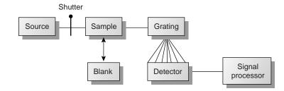
**Figure 10.27**Block diagram for a diode array spectrophotometer.
