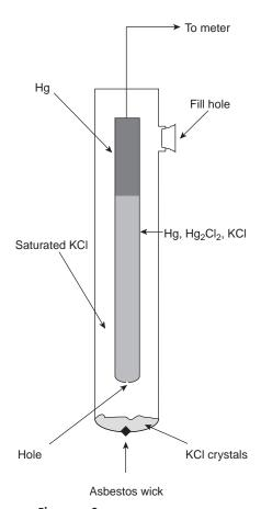
**Figure 11.8**Schematic diagram of the saturated calomel electrode (SCE).
