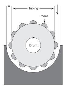
**Figure 13.20**Schematic diagram of a peristaltic pump.
