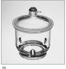
**Figure 2.9**(a) Desiccator. (b) Desiccator with stopcock for evacuating the desiccator. Photos courtesy of Fisher Scientific.
