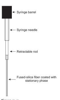
**Figure 12.19**Schematic diagram of a device for solid-phase microextractions.
