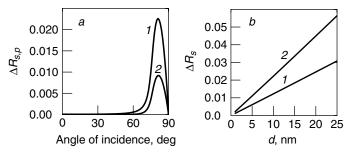
**Figure 2.15.** (a) Calculated change in substrate band intensities (1)  $\Delta R_{\rm S}$  and (2)  $\Delta R_{\rm p}$  in IRRAS of 10-nm transparent layer ( $n_2=1.5,\ k_2=0$ ) on quartz substrate as function of angle of incidence at  $\nu=1360\ {\rm cm}^{-1}$ . (b) Calculated dependence of substrate absorption depth in s-polarized spectra obtained at 80° on layer thickness;  $k_2=0,\ n_3=0.9702,\ {\rm and}\ k_3=0.013,\ n_2=(1)$  1.3 and (2)  $n_2=1.5$ .
