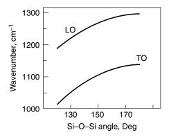
**Figure 5.3.** Frequencies of TO and LO modes calculated from Eqs. (5.3) and (5.4) versus Si-O-Si bond angle. Reprinted, by permission, from I. P. Lisovskii, V. G. Litovchenko, V. G. Lozinskii, and G. I. Steblovskii, *Thin Solid Films* **213**, 164 (1992). Copyright ⊚ 1992 Elsevier Science.
