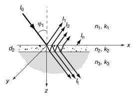
**Figure 1.12.** Scheme of beam propagation through stratified-layer system consisting of three phases. Angle of incidence of radiation is  $\varphi_1$ . Frequency-dependent optical constants of three media:  $n_1, n_2, n_3, k_1, k_2, k_3$ .
