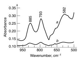
**Figure 2.49.** ATR spectra of limonite ( $Fe_2O_3 \cdot nH_2O$ , orange form/China, 5 mg): (a) with Nujol film as immersion layer; (b) measurement with dry powder. Reprinted, by permission, from U. Kunzelmann, H. Neugebauer, and A. Neckel, *Langmuir* **10**, 2444 (1994), p. 2448, Fig. 6. Copyright © 1994 American Chemical Society.
