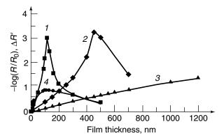
**Figure 3.14.** Band intensity measured in (1-3) absorbance and (4) reflectance  $\Delta R'$  for  $\nu_{LO}$  band of SiO<sub>2</sub> films on Al as function of film thickness in simulated IRRAS spectra. Angle of incidence is (1, 4) 80°, (2) 60°, and (3) 40°.
