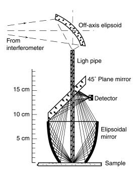
**Figure 4.19.** "Cup-on-the-saucer" optical geometry. Reprinted, by permission, from E. H. Korte and A. Otto, *Appl. Spectrosc.* **42**, 38 (1988), p. 39, Fig. 2. Copyright © 1988 Society for Applied Spectroscopy.
