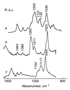
**Figure 7.42.** IR spectra of reference compounds: (a) DRIFTS of Pb(BX)<sub>2</sub> in KBr; (b) ATR of (BX)<sub>2</sub>; (c) ATR of aqueous solution of KX. Reprinted, by permission, from I. V. Chernyshova, *J. Phys. Chem. B* **105**, 8185 (2001), p. 8187, Fig. 3. Copyright ⊚ 2001 American Chemical Society.
