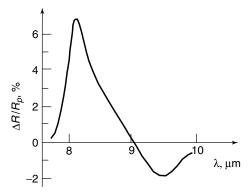
**Figure 3.31.** Simulated p-polarized IRRAS spectrum of 1-nm-thick layer of SiO<sub>2</sub> on Si, measured at  $\varphi_1 = 71^{\circ}$ . Reprinted, by permission, from V. P. Tolstoy and S. N. Gruzinov, *Opt. Spectrosc.* **71**, 77–80 (1991), p. 78, Fig. 1. Copyright © 1991 Optical Society of America.
