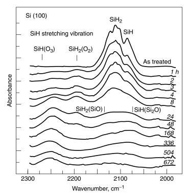
**Figure 6.24.** Absorption spectra of Si\_H stretching modes of H-terminated Si(100) surfaces after exposure to air for various times. Reprinted, by permission, from M. Niwano, J. Kageyama, K. Kinashi, J. Sawahata, and N. Miyamoto, *Surf. Sci. Lett.* **301**, L245 (1994). Copyright © 1994 Elsevier Science.
