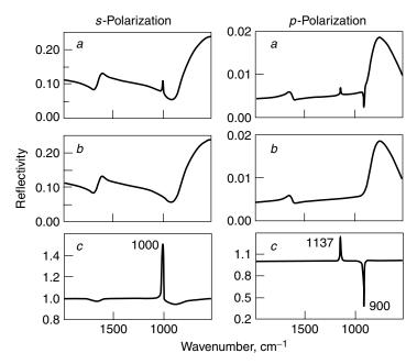
**Figure 3.27.** (a) Simulated s- and p-polarized IRRAS spectra of 10-nm film of anisotropic inorganic material (Table 3.3) at air-water (AW) interface, (b) reflection spectrum of water at  $\varphi_1 = 60^\circ$ , and (c) ratio a/b. Adapted, by permission, from K. Yamamoto and H. Ishida, Appl. Spectrosc. **48**, 775 (1994), p. 784, Fig. 12. Copyright © 1994 Society for Applied Spectroscopy.
