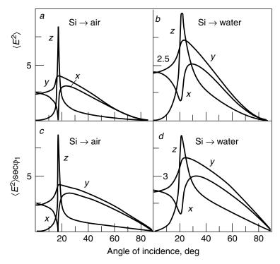
**Figure 1.19.** ATR. Influence of angle of incidence on (a,b) mean-square electric fields  $\langle E^2 \rangle$  and (c,d) normalized mean-square electric fields  $\langle E^2 \rangle \sec \varphi_1$ ; at 1000 cm<sup>-1</sup> inside model organic layer 5 nm thick  $(n_2=1.5,\ k_2=0.1)$  located at boundary of two phases:  $(a,\ c)$  Si–air;  $(b,\ d)$  Si–water. Optical constants of water and Si indicated in Table 1.1.
