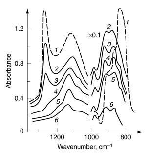
**Figure 5.34.** Variations in IR absorption spectra of  $SiO_2-Si_3N_4-SiO_x-Si$  structure after layer-by-layer chemical etching (curve number increases with decreasing film thickness). Reprinted, by permission, from Yu. A. Averkin, N. K. Karmadonov, V. A. Skryshevsky, V. I. Strikha, and A. V. Kharlamov, *Ukrainian J. Phys.* **34**, 1817, (1989). Copyright © 1989 Institute of Theoretical Physics, National Academy of Science of Ukraine.
