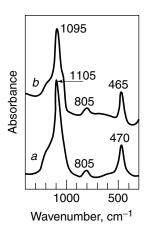
**Figure 3.55.** Experimental transmission spectra of spherical particles of amorphous  $SiO_2$  dispersed in (a) KBr ( $\varepsilon_m=2.25$ ) and (b) TICl ( $\varepsilon_m=5.1$ ). Reprinted, by permission, from J. E. Iglesias, M. Ocana, and C. J. Serna, *Appl. Spectrosc.* **44**, 418 (1990), p. 424, Fig. 9. Copyright © 1990 Society for Applied Spectroscopy.
