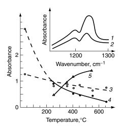
**Figure 6.1.** Effect of Ti deposition on p-polarized spectra of  $SiO_2$  interface layer recorded by IRRAS at 75° incidence: (1) before and (2) after Ti deposition. Intensities of (3) 1160-, (4) 1240-, and (5) 700-cm<sup>-1</sup> absorption bands as functions of silicon substrate temperature.
