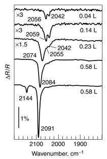
**Figure 7.4.** Spectra showing adsorption of CO on Pt(110) at 30 K. Exposures are given. Reprinted, by permission, from R. K. Sharma, W. A. Brown, and D. A. King, *Chem. Phys. Let.*, **291**, 1−6 (1998), p. 2, Fig. 1. Copyright ⊚ 1998 Elsevier Science B.V.
