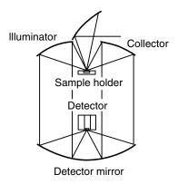
**Figure 4.27.** Optimized configuration for measuring diffuse reflectance. Reprinted, by permission, from T. Hirschfeld, *Appl. Spectrosc.* **40**, 1082−1085 (1986), p. 1083, Fig. 1. Copyright © 1986 Society for Applied Spectroscopy.
