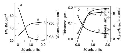
**Figure 6.7.** Dependence of (1)  $d_{SiO_2}$ , (2)  $A_{1240}/A_{1160}$ , (3)  $d_{Al_2O_3}$ , (4)  $v_{1240}$  and (5) FWHM on M.
