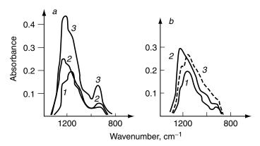
**Figure 6.15.** IRRAS spectra in *p*-polarized radiation at 75° of (a) Al-chemical oxide-InP and (b) Au-chemical oxide-InP: (1) after metal deposition; (2) after thermal annealing at 300°C for 1 h; (3) after thermal annealing at 530°C for 1 h.
