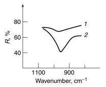
**Figure 2.32.** Experimental spectra of  $Al_2O_3$  layer on Al mirror heated at  $t=550^{\circ}C$  in air for 0.5 h, using p-polarized IRRAS at  $\varphi_1=60^{\circ}$ : (1) sample in air, (2) sample in contact with immersion medium (KRS-5). Reprinted, by permission, from V. P. Tolstoy and S. N. Gruzinov, *Opt. Spectrosc.* **63**, 489–491 (1987), p. 490, Fig. 4. Copyright © 1988 Optical Society of America.
