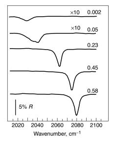
**Figure 3.36.** IRRAS spectra of various fractional coverages of CO on Ir(111) measured at 300 K. Coverages in monolayers are denoted beside each spectrum. Reprinted, with permission, from J. Lauterbach, R. W. Boyle, M. Schick, W. J. Mitchell, B. Meng, and W. H. Weinberg, *Surf. Sci.* **366**, 228 (1996), p. 228, Fig. 2. Copyright © 1996 Elsevier Science Ltd.
