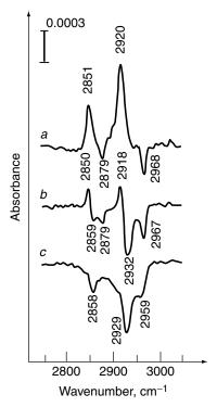
**Figure 3.90.** IRRAS spectra of (a) SAM of tetradecyltrichlorosilane (TTS) prepared in dry inert-gas atmosphere, (b) partly disordered film of TTS prepared in ambient atmosphere, and (c) liquid film of paraffin oil ( $d \approx 10\text{Å}$ ) on silicon substrates (p-polarization,  $80^{\circ} \pm 3^{\circ}$  incidence). Reprinted, by permission, from H. Hoffmann, U. Mayer, and A. Krischanitz, *Langmuir* **11**, 1304 (1995), p. 1311, Fig. 7. Copyright © 1995 American Chemical Society.
