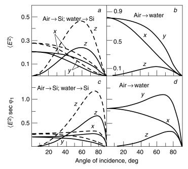
**Figure 1.15.** External reflection. Influence of angle of incidence on (a, b) mean-square electric fields  $\langle E^2 \rangle$  and (c, d) normalized mean-square electric fields  $\langle E^2 \rangle$  sec  $\varphi_1$  at  $1000 \text{ cm}^{-1}$  inside model organic layer 5 nm thick  $(n_2=1.5 \text{ and } k_2=0.1)$  located at boundaries: (a, c) air–Si (solid line) and water–Si (dashed line) and (b, d) air–water. Optical constants of water and Si indicated in Table 1.1.
