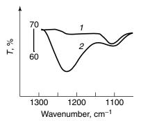
**Figure 2.27.** Experimental transmission spectrum of 1.4-nm SiO<sub>2</sub> layer on Si. Measurements were performed for p-polarization and angle of incidence  $\varphi_1 = 60^\circ$ : (1)  $n_1 = n_3 = 1.0$ , (2)  $n_1 = n_3 = 2.37$ . Reprinted, by permission, from V. P. Tolstoy and S. V. Habibova, *Vestnilk Leningradskogo Universiteta. Phizika, Khimia* **2** 106 (1989), p. 109, Fig. 4 Copyright © 1989 St. Petersburg University Press.
