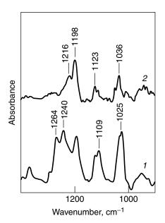
**Figure 2.52.** Comparison of (1) in situ ATR and (2) ex situ DRIFTS spectra of same chalcopyrite sample <30  $\mu$ m size contacted with ethyl xanthate solution of pH 9.5 of  $7.6 \times 10^{-4}$  M. Baseline correction was done for both reflection spectra. Adaptated, by permission, from J. A. Mielczarski, J. M. Cases, and O. Barres, *J. Colloid Interface Sci.* **178**, 740 (1996), p. 744, Fig. 5. Copyright © 1996 Academic Press.
