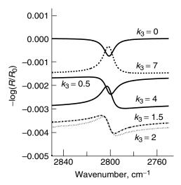
**Figure 3.29.** Dependence of band shape in *p*-polarized IRRAS spectrum of hypothetical organic layer 1 nm thick on absorption index of substrate with  $n_3=3.4$ . Absorption indices are indicated. Dielectric function of film was specified by S=0.001,  $\gamma=10~{\rm cm}^{-1}$ ,  $\nu_0=2800~{\rm cm}^{-1}$ , and  $\varepsilon_\infty=1.7$ ;  $\varphi_1=80^\circ$ .
