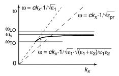
**Figure 3.6.** Dispersion curves of surface polariton (solid line) at interface of inactive and active media characterized by  $\varepsilon_1$  and  $\varepsilon_2$ , respectively. Short-dashed line: dispersion line of incident photon in inactive medium with  $\varepsilon_1$ ; long-dashed line: in ATR prism with  $\varepsilon_{pr} > \varepsilon_1$ .
