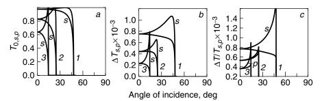
**Figure 2.4.** Dependence of s- and p-polarized (a) transmittance  $T_{0,s,p}$ , (b) absorption depth  $\Delta T_{s,p}$ , and (c) transmissivity  $\Delta T/T_{s,p}$  on angle of incidence of IR radiation for different refractive indices of input medium (=substrate): (1)  $n_1 = 1.35$ , (2)  $n_1 = 2.4$ , and (3)  $n_1 = 4.0$ ;  $d_2 = 1$  nm,  $n_2 = 1.564$ ,  $k_2 = 0.384$ ,  $\nu = 1200$  cm<sup>-1</sup>,  $n_3 = 1$ .
