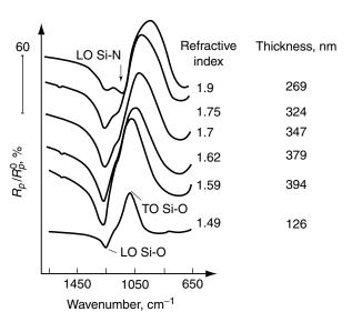
**Figure 5.13.** The p-polarized IRRAS spectra at  $70^{\circ}$  of various  $SiO_xN_y$  thin films on Si wafer. Refractive indices are shown on right of spectra;  $R_p$  of bare silicon wafer in p-polarization is used as references. Reprinted, by permission, from M. Firon, C. Bonnelle, and A. Mayeux, *J. Vac. Sci. Technol. A* **14**, 2488 (1996). Copyright © 1996 American Vacuum Society.
