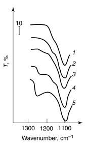
**Figure 4.2.** Multiple-transmission IR spectra of SiO<sub>2</sub> layers on silicon surface,  $\varphi_1 = \varphi_B = 74^\circ$ : (1) after etching 1 min in HF; and after annealing in air at (2) 200, (3) 240, (4) 400, and (5) 500° C. Reprinted, by permission, from V. P. Tolstoy, L. P. Bogdanova, and V. B. Aleskovski, *Doklady AN USSR* **291**, 913 (1986), p. 914, Fig. 2. Copyright © 1986 Doklady AN USSR.
