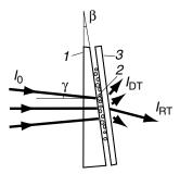
**Figure 4.24.** Cuvette for measuring DT spectra of powders: (1) ZnSe wedge-shaped window; (2) powder sample; (3) plane-parallel window. Reprinted, by permission, from S. P. Scherbakov, E. D. Kriveleva, V. P. Tolstoy, and A. I. Somsikov, *Pribory i tekhnika experimenta* No. 1, 206–208 (1992), p. 206, Fig. 1. Copyright © 1992 Pribory i tekhnika experimenta.
