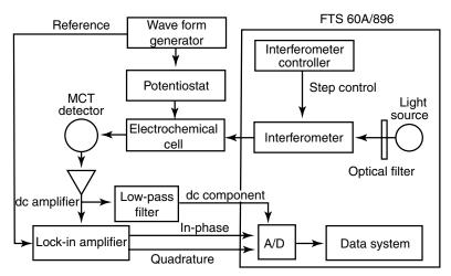
**Figure 4.56.** Block diagram for experimental setup for potential modulated FTIR measurements. Reprinted, by permission, from K. Ataka, Y. Hara, and M. Osawa, *J. Electroanal. Chem.* **473**, 34 (1999), p. 36, Fig. 1. Copyright © 1999 Elsevier Science S.A.
