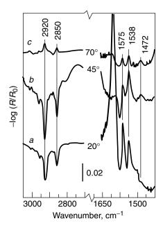
**Figure 2.13.** Reflection spectra of calcite after incubation for 5 min in  $3.3 \times 10^{-5}$  *M* oleate solution, pH 10, recorded for *p*-polarization at angles of incidence of (a)  $20^{\circ}$ , (b)  $45^{\circ}$ , and (c)  $70^{\circ}$ . Reprinted, by permission, from J. A. Mielczarski and E. Mielczarski, *J. Phys. Chem. B* **103**, 5852 (1999), p. 5856, Fig. 7. Copyright © 1999 American Chemical Society.
