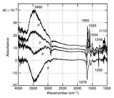
**Figure 3.65.** ATR-SEIRA spectra from uracil on Au electrode at various potentials in 10 mM uracil  $+0.1 M \text{ LiCIO}_4$  solution: (a) +0.3 V, (b) +0.6 V, (c) +0.7 V, (d) +0.9 V. Reference potential is +0.20 V (Ag/AgCl). Positive peaks correspond to increase in absorption at sample potential. Reprinted, by permission, from M. Futamata and D. Diesing, *Vib. Spectrosc.* **19**, 187–192 (1999), p. 190, Fig. 3. Copyright © 1999 Elsevier Science B.V.
