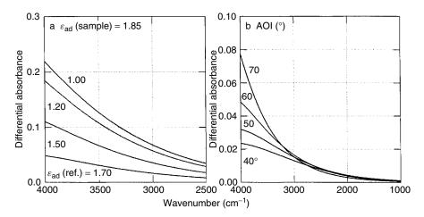
**Figure 3.66.** Theoretical IR background shift in ATR-SEIRA spectra as function of (a) dielectric constant of adsorbate layer without chemisorption [ $\varepsilon_{ads}$ (ref)] at incident angle of 60° and (b) angle of incidence (AOI). Dielectric constant of adsorbate layer under chemisorption  $\varepsilon_{ads}$  (sample) is 1.85. Reprinted, by permission, from M. Futamata, *Chem. Phys. Lett.* **333**, 337-343 (2001), p. 342, Fig. 5a. Copyright © 1999 Elsevier Science B.V.
