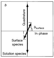
**Figure 3.50.** Projection of solution and surface bands into in-phase and quadrature channels (a) before and (b) after phase rotation.
