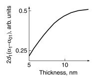
**Figure 6.12.** Experimental dependence of  $2d_1(\alpha_1 - \alpha_{01})$  on  $d_{Au}$  for Au–SiO<sub>2</sub>–Si structure.
