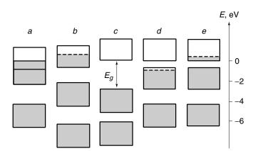
**Figure 1.2.** Schematic representation of band structure of (a, b) metals (overlapping bands and partially filled band); (c) insulators; (d, e) p- and n- degenerate semiconductors. Here,  $E_g$  is width of band gap and dash line indicates position of Fermi level.
