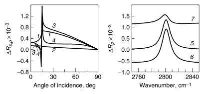
**Figure 2.37.** Angular dependence of quantities (1, 2)  $\Delta R_{\rm S}$  and (3, 4)  $\Delta R_{\rm p}$  for ATR spectrum of organic layer in Ge–Ag–organic layer structure (Kretschmann geometry) and (5–7) spectrum  $\Delta R_{\rm p}$  of this layer calculated for  $\varphi_1=15^\circ:n_1=4.0;\ d_{\rm Ag}:\ (1,\ 3,\ 5)\ 0,\ (6)\ 3,\ (2,\ 4,\ 7)\ 12\ {\rm nm};\ n_{\rm Ag}=1.94,\ k_{\rm Ag}=22.1,\ d_{\rm 3}=1\ {\rm nm},\ n_{\rm 3}=1.52,\ k_{\rm 3}=0.12,\ n_{\rm 4}=1,\ \nu=2800\ {\rm cm}^{-1}.$
