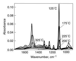
**Figure 7.11.** Single-reflection IRRAS of imidazole film on Cu under vacuum at series of temperatures as film is heated from room temperature to 325°C in 50°C increments. Film was held at each temperature for 15 min before increasing temperature. Reprinted, by permission, from R. L. Opila, H. W. Krautter, B. R. Zegarski, and L. H. Dubois, *J. Electrochem. Soc.* **142**, 4074–4077 (1995), p. 4075, Fig. 3. Copyright © 1999 Electrochemical Society.
