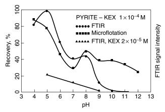
**Figure 7.28.** Dependence of FTIR signal intensity and microflotation recovery on pH for pyrite in potassium ethyl xanthate (KEX) solution of  $1 \times 10^{-4} \, M$  and FTIR signal intensity in KEX solution of  $2 \times 10^{-5} \, M$ . Full length of intensity axis corresponds to 1.0% absorption. Reprinted, by permission, from J. O. Leppinen, *Int. J. Miner. Process.* **30**, 245 (1990), p. 254, Fig. 7. Copyright © 1990 Elsevier Publishers B.V.
