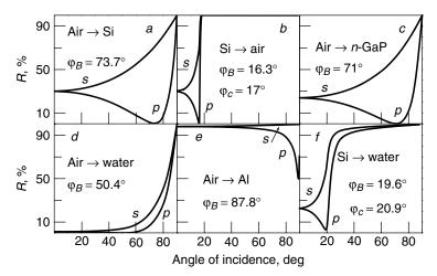
**Figure 1.11.** Influence of angle of incidence on reflectance at 1000 cm<sup>-1</sup> for boundary of two phases: (a) air–Si; (b) Si–air; (c) air–n-GaP; (d) air–water; (e) air–Al; (f) Si–water. Optical constants are indicated in Table 1.1.
