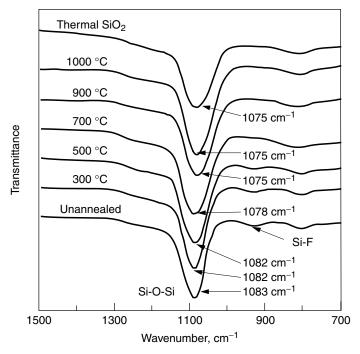
**Figure 5.7.** FTIR transmission spectra of LPD  $F_x$ SiO<sub>y</sub> oxide at different annealing temperatures. Reprinted, by permission, from C.-F. Yeh and C.-L. Chen, *J. Electrochem. Soc.* **142**, 3579 (1995). Copyright © 1995 Electrochemical Society, Inc.
