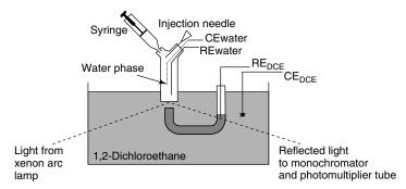
**Figure 4.17.** Experimental set-up employed in SEC measurements at liquid-liquid interface. CE refers to counter electrode and RE to reference electrode for two phases. Reprinted, by permission, from Z. Ding, R. G. Wellington, P. -F. Brevet, and H. H. Girault, *J. Electroanal. Chem.* **420**, 35 (1997). p. 37, Fig. 1. Copyright © 1997 Elsevier Science B.V.
