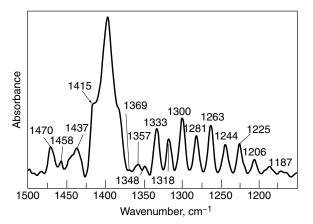
**Figure 3.77.** DRIFTS spectra of stearic acid ( $C_{18}$ ) self-assembled on silver 2- $\mu$ m particles in region of 1100–1500 cm<sup>-1</sup>. Reprinted, by permission, from S. J. Lee and K. Kim, *Vib. Spectrosc.* **18**, 187 (1998), p. 192, Fig. 2. Copyright © 1998 Elsevier Science B.V.
