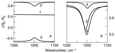
**Figure 2.29.** Spectra of (1)  $R_{0,p}$ , (2, 4-6)  $R_p$ , and (3)  $\Delta R_p$  of 80-nm layer characterized by oscillator parameters  $\varepsilon_{\infty}=2.3$ ,  $\gamma=15$  cm<sup>-1</sup>,  $\nu_0=1200$  cm<sup>-1</sup>, S=0.015 and located at germanium-aluminum interface ( $n_1=4.0$ , n and k of Al from Ref. [75]); (a)  $\varphi_1=85^{\circ}$ , (b)  $\varphi_1$ : (4)  $85^{\circ}$ , (5)  $30^{\circ}$ , and (6)  $60^{\circ}$ .
