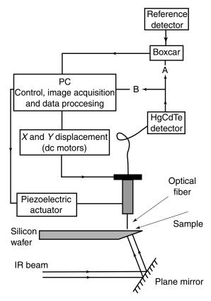
**Figure 4.39.** Experimental set-up for scanning near-field optical microscopy (SNOM) in IR range. Reprinted, by permission, from A. Piednoir, C. Licoppe, and F. Creuzet, *Opt. Commun.* **129**, 414–422 (1996), p. 415, Fig. 1. Copyright © 1996 Elsevier Science B.V.
