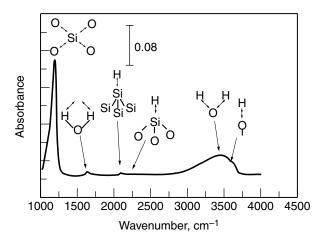
**Figure 6.18.** Typical MIT IR spectrum of two hydrophilic Si(111) wafers bonded at room temperature. Reprinted, by permission, from M. K. Weldon, V. E. Marsico, Y. J. Chabal, D. R. Hamann, S. B. Christman, and E. E. Chaban, *Surf. Sci.* **368**, 163 (1996). Copyright ⊚ 1996 Elsevier Science.
