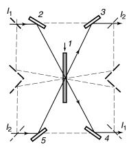
**Figure 4.5.** Schematic arrangement for studying uniformity in film: (1) plate, which can be moved with an electromechanical drive; (2–5) mirrors. Reprinted, by permission, from V. P. Tolstoy, *Methods of UV-Vis and IR Spectroscopy of Nanolayers*, St. Petersburg University Press, St. Petersburg, 1998, p. 130, Fig. 4.9. Copyright © St. Petersburg University Press.
