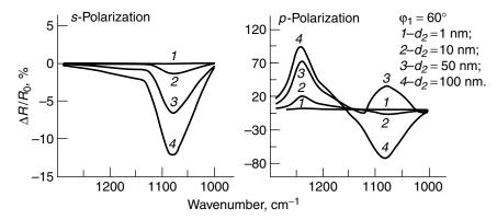
**Figure 3.19.** Simulated s- and p-polarized IRRAS spectra of  $SiO_2$  layers on Si as function of layer thickness at  $\varphi_1 = 60^\circ$ . Optical constants of thermal  $SiO_2$  are specified according to Ref. [52];  $n_3 = 3.42$ .
