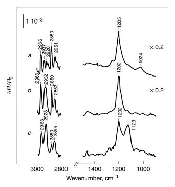
**Figure 7.24.** Experimental spectra from IRRAS of octyl xanthate (OX) adsorbed on gold. Concentrations and adsorption times are (a) 1 mM and 10 min, (b) 10  $\mu$ M and 10 min, and (c) 1 $\mu$ M and 10 min. Reprinted, by permission, from A. Ihs, K. Uvdal, and B. Liedberg, *Langmuir* 9, 733 (1993), p. 736, Fig. 5. Copyright © 1993 American Chemical Society.
