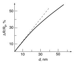
**Figure 2.11.** Dependence of reflectivity  $\Delta R/R$  on thickness d of SiO<sub>2</sub> layer on Si for p-polarized radiation ( $v=1240~{\rm cm^{-1}},~n_3=3.42,~\varphi_1=60^\circ$ ). Dashed line is tangent to reflectivity curve. Reprinted, by permission, from S. N. Gruzinov and V. P. Tolstoy, *Zhurnal prikladnoi spektroskopii* **46**, 775 (1987), p. 777, Fig. 2 Copyright © 1987 "Nauka i tekhnika".
