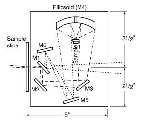
**Figure 4.26.** Schematic layout of Perkin-Elmer PEDR accessory:  $M_1$  — double-sided mirror;  $M_2$ ,  $M_3$ ,  $M_5$ ,  $M_6$  — plane mirrors;  $M_4$  — ellipsoidal mirror. Courtesy of Perkin-Elmer, Inc.
