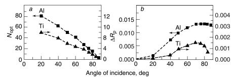
**Figure 2.8.** Dependence on angle of incidence of (a) optimum number of reflections  $N_{\rm opt}$  and (b) absorption depth  $\Delta R_p$  for  $N_{\rm opt}$  reflections for 1-nm layer  $(\hat{n}_3 = 1.564 - 0.384i)$  at Al  $(\hat{n}_3 = 18.6 - 77i)$  and Ti  $(\hat{n}_3 = 6.5 - 14.8i)$  substrate; v = 1200 cm<sup>-1</sup>; p-polarization.
