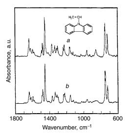
**Figure 7.49.** Spectra measured by IRRAS of (a) isotropic NVCz film and (b) vapor deposition polymerization (VDP) film deposited at substrate temperature of 255 K. Reflection spectrum of isotropic NVCz film was obtained by KK transformation of transmission absorption spectrum of KBr composite containing intrinsic NVCz. Reprinted, by permission, from M. Tamada, H. Koshikawa, and H. Omichi, *Thin Solid Films* **292**, 164 (1997) p. 165, Fig. 2. Copyright ⊚ 1997 Elsevier Science S.A.
