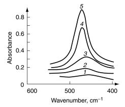
**Figure 5.26.** The p-polarized absorption spectra of CaF<sub>2</sub> layers on Si substrates at 75° incidence for different thicknesses: (1) 30, (2) 45, (3) 100, (4) 330, and (5) 460 nm.
