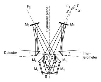
**Figure 4.28.** Optical diagram of Praying Mantis (Harrick Scientific Inc.) diffuse-reflectance accessory:  $M_1$ ,  $M_2$ ,  $M_5$ ,  $M_6$  — plane mirrors;  $M_3$ ,  $M_4$  —  $6:1\,90^\circ$  off-axis focusing and collecting ellipsoids. Sample is placed at position S. Adapted, by permission, from K. Moradi, C. Depecker, and J. Corset, *Appl. Spectrosc.* **48**, 1491 (1994), p. 1492, Fig. 2. Copyright © 1994 Society for Applied Spectroscopy.
