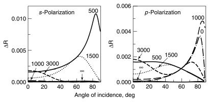
**Figure 2.18.** Calculated s- and p-polarized absorption depth of 1-nm upper layer on BML substrate,  $\Delta R$ , as function of angle of incidence for different thicknesses (in nm) of buffer layer. Optical constants of system are as in Fig. 2.17. Curves for film on bare metal and transparent substrates are labeled with thickness 0 and  $\infty$ , respectively.
