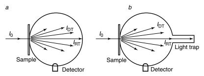
**Figure 4.21.** Measurement of (a) total and (b) diffuse transmittance with integrating sphere.  $I_{RT}$  and  $I_{DT}$  are regularly and diffusively transmitted radiation, respectively.
