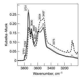
**Figure 7.1.** DRIFTS spectra of  $\gamma$ -alumina calcined at 700°C for 1 h under flowing N<sub>2</sub> before pyridine adsorption (dark solid line), after pyridine adsorption at room temperature (dash line), and after pyridine adsorption followed by heating at 400°C for 1 h (dotted line). All spectra recorded at room temperature. Adapted, by permission, from X. Liu and R. E. Truitt, *J. Am. Chem. Soc.* **119**, 9856 (1997), p. 9860, Fig. 4a. Copyright © 1997 American Chemical Society.
