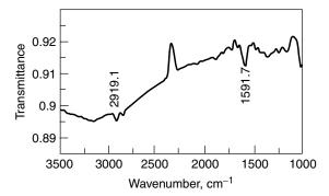
**Figure 7.51.** FTIR spectrum of steel surface after failure of steel−ethylene-vinyl acetate assembly. Reprinted, by permission, from S. Bistac, M. F. Vallat, and J. Schultz, *Appl. Spectrosc.* **51**, 1823 (1997), p. 1824, Fig. 2. Copyright ⊚ 1997 Society for Applied Spectroscopy.
