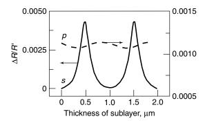
**Figure 2.17.** Calculated reflectivity of upper layer,  $\Delta R/R'$ , for s- and p-polarized radiation as function of thickness of lower layer,  $d_3$ , at  $\varphi_1=60^\circ$ ,  $\lambda=3$  µm, for  $d_2=1$  nm,  $n_2=1.3$ ,  $k_2=0.1$ ,  $n_3=1.7$ ,  $k_3=0$ ,  $n_4=3.2$ ,  $k_4=23$ . Reprinted, by permission, from V. P. Tolstoy and E. Yu. Egorova, *Opt. Spectrosc.* **68**, 663–647 (1990), p. 663, Fig. 1. Copyright © 1990 Optical Society of America.
