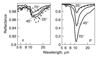
**Figure 3.59.** Experimental (solid lines) and calculated (dashed lines) IRRAS spectra of porous anodic alumina film 500 nm thick on AI, measured at three different angles of incidence with s-and p-polarized radiation. Calculation was performed using experimentally derived refractive index. Reprinted, by permission, from E. Wackelgard, *J. Phys. Condens. Matter* **8**, 4289 (1996), p. 4294, Fig. 2. Copyright © 1996 IOP Publishing Ltd.
