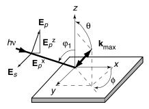
**Figure 3.82.** Definition of Euler angles describing orientation and principal components of maximum absorption index vector,  $\mathbf{k}_{\text{max}}$ .
