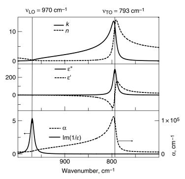
**Figure 1.1.** Frequency dependences of n, k,  $\varepsilon'$ ,  $\varepsilon''$ , and  $\text{Im}(1/\hat{\varepsilon})$  for  $\beta$ -SiC characterized by S=3.3,  $\varepsilon_\infty=6.7$ ,  $\gamma=8.49~\text{cm}^{-1}$ , and  $\nu_0=793.6~\text{cm}^{-1}$ . Also shown are optical transverse and longitudinal frequencies ( $\nu_{\text{TO}}$  and  $\nu_{\text{LO}}$ , respectively).
