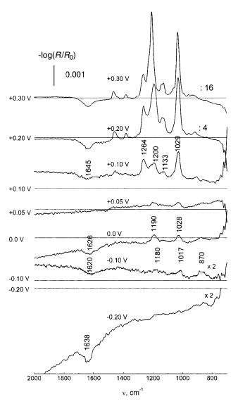
**Figure 7.43.** Unpolarized difference ATR spectra of galena electrode–electrolyte interface at potentials starting at -0.5 V. Electrolyte is  $1 \times 10^{-3}$  M potassium n-butyl xanthate solution in 0.05 M borate buffer (pH 9.18) at N<sub>2</sub> atmosphere. Other conditions as in Fig. 7.41. Reprinted, by permission, from I. V. Chernyshova, J. Phys. Chem. B **105**, 8185 (2001), p. 8189, Fig. 5. Copyright © 2001 American Chemical Society.
