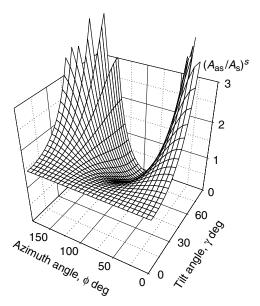
**Figure 3.88.** Dependence of ratio of peak intensities of  $v_{as}CH_2$  and  $v_sCH_2$  bands in *s*-polarized IRRAS spectra,  $(A_{as}/A_s)^s$ , of biaxial monolayer on quartz on tilt and azimuth angles,  $k_{max,as}/k_{max,s} = 1.5$ . Adapted, by permission, from I. V. Chernyshova and K. Hanumantha Rao, *J. Phys. Chem. B* **105**, 810 (2001), p. 816, Fig. 9. Copyright © 2001 American Chemical Society.
