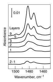
**Figure 3.80.** ATR spectra in  $CH_2$  scissoring region of one-, two-, three-, five-, and nine-layer LB films of stearic acid on germanium. Adapted, by permission, from F. Kimura, J. Umemura, and T. Takenaka, *Langmuir* **2**, 96 (1986), p. 98, Fig. 5. Copyright © 1986 American Chemical Society.
