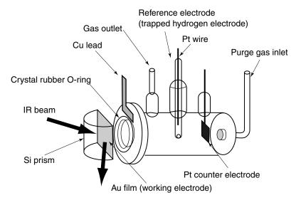
**Figure 4.49.** SEC reflection cell with thin-layer (20-nm Au) electrode. Reprinted, by permission, from K. Ataka, T. Yotsuyanagi, and M. Osawa, *J. Phys. Chem.* **100**, 10664 (1996), p. 10665, Fig. 1. Copyright © 1996 American Chemical Society.
