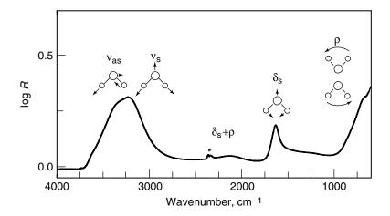
Figure 1.4. ATR spectrum of water. Asterisk indicates atmosphere CO<sub>2</sub> absorption.
