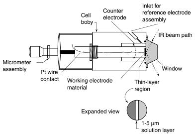
**Figure 4.46.** Schematic diagram of SEC reflection cell with Dove prism window. Slice through center of cell viewed from top is shown. Expanded view of thin-layer cavity region also appears. Reprinted, by permission, from C. Korzeniewski and M. W. Severson, *Spectrochim. Acta A* **51**, 499 (1995), p. 501, Fig. 1. Copyright © 1995 Elsevier Science Ltd.
