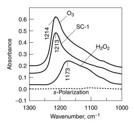
**Figure 5.10.** S-(dashed line) and *p*-(solid lines) polarized absorption spectra of native silicon oxide formed by several methods. Reprinted, by permission, from T. Ohwaki, M. Takeda, and Y. Takai, *Jpn. J. Appl. Phys.* **36**, 5507 (1997). Copyright © 1997 Publication Board of Japanese Journal of Applied Physics.
