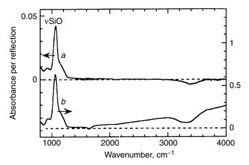
**Figure 3.48.** Surface roughening of p-Si during anodic dissolution in transpassivation regime Electrolyte is 1 M NH<sub>4</sub>Cl + 0.025 M HF + 0.025 M NH<sub>4</sub>F. Potential (a) +5 V (slow electropolishing) and (b) +40 V (transpassivation). Reprinted, by permission, from J. N. Chazalviel, B. H. Erne, F. Maroun, and F. Ozanam, J. Electroanal. Chem. **502**, 180–190 (2001), p. 188, Fig. 9. Copyright © 2001 Elsevier Science B.V.
