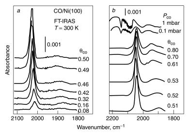
**Figure 7.3.** Series of IR spectra for increasing CO coverages above 0.5 ML on Ni(100) at 300 K. Upper two spectra display rotational fine structure of gas phase CO. Reprinted, by permission, from A. Grossman, W. Erley, and H. Ibach, *Surface Science*, **330**, L646−L650 (1995), p. L647, Fig. 1. Copyright ⊚ 1995 Elsevier Science B.V.
