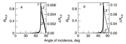
**Figure 2.35.** Dependence on angle of incidence of (1) reflecance  $R_0$  for (a) quartz–hexafluorobenzene interface and (b) Ge–amorphous Si interface and of absorption depths (2)  $\Delta R_s$  and (3)  $\Delta R_p$  for layer at given interfaces;  $n_2 = 1.3$ ,  $k_2 = 0.1$ ,  $d_2 = 1$  nm, v = 2800 cm<sup>-1</sup>, (a)  $n_1 = 1.402$ ,  $n_3 = 1.351$ , (b)  $n_1 = 4.03$ ,  $n_3 = 3.84$ .
