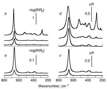
**Figure 3.13.** Simulated *p*-polarized IRRAS spectra of  $\alpha$ -Fe<sub>2</sub>O<sub>3</sub> layers on Fe in (a,b) the absorbance and (c,d)  $\Delta R$  units,  $\varphi_1=75^\circ$ . Layer thickness increases from lower to upper curve in series: (a,c) 10 and 50 nm and (b,d) 100, 150, and 500 nm. Parameters of Maxwell-Helmholtz-Drude formula (1.46) for  $\alpha$ -Fe<sub>2</sub>O<sub>3</sub> listed in Table 3.2.
