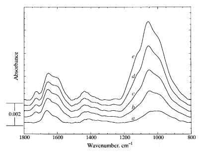
**Figure 7.9.** Series of IRRAS spectra on copper in air containing 80% relative humidity (RH) and 8.7 ppm SO<sub>2</sub>. Exposure time (a) 1, (b) 4, (c) 8, (d) 12, and (e) 16 h. Reprinted, by permission, from J. Itoh, T. Sasaki, T. Ohtsuka, and M. Osawa, *J. Electroanal. Chem.* **473**, 256−264 (1999), p. 259, Fig. 3. Copyright ⊚ 1999 Elsevier Science S.A.
