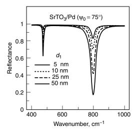
**Figure 5.30.** The *p*-polarized IRRAS spectra of SrTiO<sub>3</sub>-Pd-Si recorded at 75° angle of incidence for different SrTiO<sub>3</sub> film thicknesses. Reprinted, by permission, from H. Myoren, T. Matsumoto, and Y. Osaka, *Jpn. J. Appl. Phys.* **31**, L1425 (1992). Copyright ⊚ 1992 Publication Board Japanese Journal of Applied Physics.
