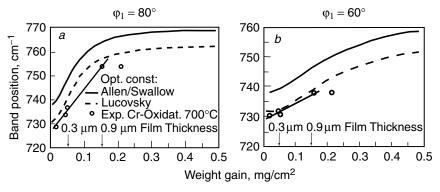
**Figure 3.15.** Position of  $\nu_{LO}$  band in experimental (circles) and calculated (lines) IRRAS of spectra  $Cr_2O_3$  films on Ni as function of film thickness. Angle of incidence is (a)  $80^{\circ}$  and (b)  $60^{\circ}$ . Theoretical curves were generated using Eq. (3.26) and different optical constants of  $Cr_2O_3$ . Reprinted, by permission, from Th. Scherubl and L. K. Thomas, *Appl. Spectrosc.* **51**, 844 (1997), p. 847, Fig. 3. Copyright © 1997 Society for Applied Spectroscopy.
