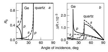
**Figure 2.23.** Angle-of-incidence dependence of (a) reflectance  $R_0$  of quartz IRE-air and Ge IRE-air interfaces and (b) absorption depth  $\Delta R$  of layer with  $n_2=1.3$ ,  $k_2=0.1$ , and  $d_2=1$  nm at these interfaces;  $n_{\rm quartz}=1.402$ ,  $n_{\rm Ge}=4.03$ . In all cases,  $n_3=1$ ,  $\nu=2800$  cm<sup>-1</sup>.
