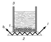
Figure 4.33. Cell for recording ATR spectra of the powder–liquid interface: (1) powder; (2) IRE, (3) cuvette.
