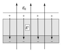
Figure 3.4. Polarization of slab in external electrostatic electric field E<sub>0</sub> perpendicular to slab.
