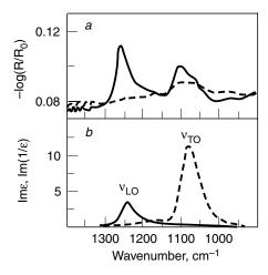
**Figure 3.1.** (a) Experimental transmission of two thermal SiO<sub>2</sub> layers 26 nm thick each produced on both sides of Si plate by heating in air at 800°C for 20 min: s- (dashed line) and p-polarization (solid line);  $\varphi_1 = 74^\circ$ . (b) The LO (solid line) and TO (dashed line) energy loss functions calculated on basis of optical constants of thermal Si dioxide grown at 1150°C [52].
