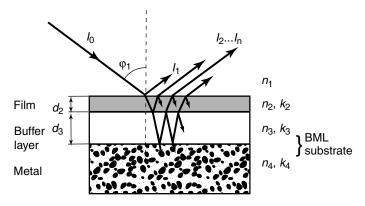
Figure 2.16. Schematic diagram of film on BML (interference) substrate.
