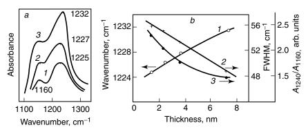
**Figure 5.18.** (a) IRRAS of anodic oxide SiO<sub>2</sub> grown on a-Si:H layer for various SiO<sub>2</sub> thicknesses d: (1) 1.5, (2) 3.6, and (3) 7.2 nm. (b) Various spectral parameters as function of oxide layer thickness d: (1)  $\nu_m$ , (2) FWHM(1240), and (3)  $A_{1240}/A_{1160}$ . Reprinted, by permission, from V. A. Skryshevsky, V. I. Strikha, and H. Gleskova, *Czech J. Phys.* **42**, 331 (1992). Copyright © 1992 Czech Journal of Physics.
