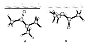
**Figure 7.48.** Schematic diagram indicating orientation of dimethylacetamide at positively charged metal electrode (a) and at negatively charged electrode (b). Reprinted, by permission, from W. R. Fawcett, A. A. Kloss, J. J. Calvente, and N. Marinkovic, *Electrochim. Acta* **44**, 881 (1998), p. 883, Fig. 2. Copyright © 1998 Elsevier Science Ltd.
