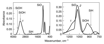
**Figure 5.5.** IR absorption of (1) CVD oxide (SiH<sub>4</sub> with 60% concentrated  $H_2O_2$ ) and (2) thermal oxide produced using  $O_2$  at  $1050^{\circ}$ C. Reprinted, by permission, from F. Gaillard, P. Brault, and P. Brouquet, *J. Vac. Sci. Technol. A* **15**, 2478 (1997). Copyright © 1997 American Vacuum Society.
