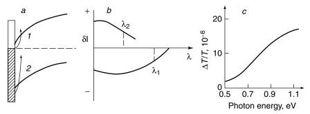
**Figure 6.21.** (a) Scheme of electronic transitions; (b) general shapes of IR absorption for surface with *n*-type conduction; (c) absorption of defects of trivalent silicon in SiO<sub>2</sub>-Si.
