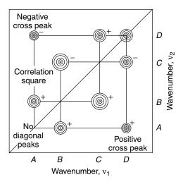
**Figure 3.52.** Schematic contour map of asynchronous 2DIR correlation spectrum. Shaded areas represent negative-intensity regions. Reprinted, by permission, from I. Noda, A. E. Dowrey, and C. Marcott, *Appl. Spectrosc.* **47**, 1317 (1993), p. 1318, Fig. 3. Copyright © 1993 Society for Applied Spectroscopy.
