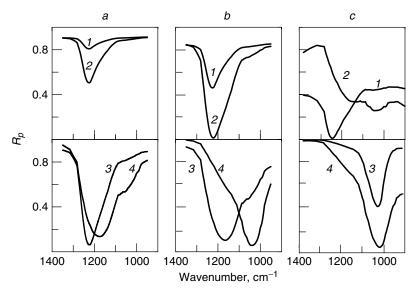
**Figure 2.31.** Calculated *p*-polarized IRRAS spectra of SiO<sub>2</sub> layer of thickness (1) 1, (2) 5, (3) 20, and (4) 100 nm located at Ge\_Al interface. Spectra were obtained for  $\varphi_1$  values of (a) 30°, (b) 60°, and (c) 85°. Optical constants of SiO<sub>2</sub> were specified in Ref. [2] and of Al in Ref. [75],  $n_{\text{Ge}} = 4.0$ .
