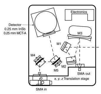
**Figure 4.18.** Optical layout of fiber-optics interface (Nicolet Instrument Inc.). Reprinted, by permission, from M. J. Smith and T. E. May, *Am. Lab.*, February 1992, p. RP-51. Copyright © 1992 Nicolet Instrument Corp.
