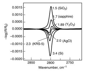
**Figure 3.28.** Band shape in *p*-polarized IRRAS spectra of hypothetical organic layer 1 nm thick as function of refractive index  $n_3$  of transparent substrate (indicated in figure). Dielectric function of film was specified by S = 0.001,  $\gamma = 10$  cm<sup>-1</sup>,  $\nu_0 = 2800$  cm<sup>-1</sup>, and  $\varepsilon_{\infty} = 1.7$ ;  $\varphi_1 = 83^{\circ}$ .
