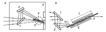
**Figure 4.4.** Schematic diagram of multipurpose accessory. Arrangement for recording (a) single-, double- and (b) multiple-transmission spectra: (1, 2) guiding mirrors; (3) plateau; (4) sample; (5) directing mirrors. Reprinted, by permission, from V. P. Tolstoy, *Methods of UV-Vis and IR Spectroscopy of Nanolayers*, St. Petersburg University Press, St. Petersburg, 1998, p. 128, Fig. 4.8. Copyright © St. Petersburg University Press.
