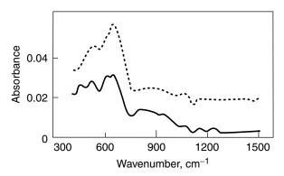
**Figure 5.29.** IR absorbance spectra of as-deposited 84-nm  $Ta_2O_5$  film on Si wafer measured at normal incidence (dashed line) and  $65^{\circ}$  angle of incidence (solid line). Reprinted, by permission, from R. A. B. Devine, *Appl. Phys. Lett.* **68**, 1924 (1996). Copyright © 1996 American Institute of Physics.
