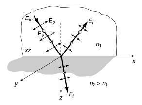
Figure 1.9. Electric field vectors in two-phase system.
