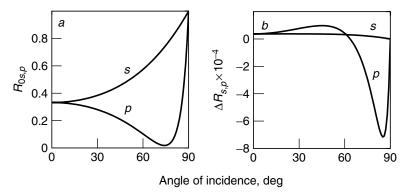
**Figure 2.12.** Dependences of (a) reflectance of bare substrate and (b) absorption depth of 1-nm model film ( $n_2=1.3, k_2=0.1$ ) measured by transparent IRRAS with s- and p-polarization on angle of incidence  $\varphi_1$ :  $n_1=1, n_3=3.4, k_3=1, \nu=3000 \text{ cm}^{-1}$ .
