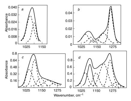
**Figure 5.2.** Result of deconvolution into Gaussian profiles of stretching absorption band of SiO<sub>2</sub> films 27 nm (a,b) and 600 nm (c,d) thick. Band was recorded at  $\varphi=0^{\circ}$  (a,c) and in p-polarized light at  $\varphi=75^{\circ}$  (b,d).
