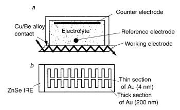
**Figure 4.48.** (a) Schematic diagram of SEC cell with multiple-reflection IRE. (b) Top view of patterned Au–ZnSe IRE electrode by Bae et al. [417]. Numbers in parentheses are thicknesses of Au deposits in two sections.
