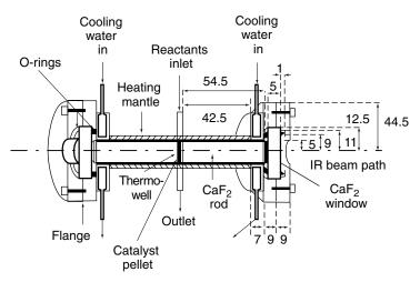
**Figure 4.40.** The IR reactor cell for transmission measurements (all dimensions in millimeters). Reprinted, by permission, from S. S. C. Chuang, M. A. Brundage, M. W. Balakos, and C. Srinivas, *Appl. Spectrosc.* **49**, 1151–1163 (1995), p. 1152, Fig. 1. Copyright © 1995 Society for Applied Spectroscopy.
