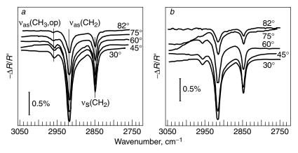
**Figure 2.19.** BML-IRRAS spectra of SAM of OTS on Si\_CoSi<sub>2</sub>\_Si substrate with 200-nm buffer layer as function of angle of incidence: (a) *p*-polarization, (b) *s*-polarization. Reprinted, by permission, from Y. Kobayashi and T. Ogino, *Appl. Surf. Sci.* **100/101**, 407 (1996), p. 409, Fig. 2. Copyright ⊚ 1996 Elsevier Science B.V.
