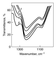
**Figure 6.8.** *p*-polarized IR transmission spectra at  $\varphi = 75^{\circ}$  of PSG for different phosphorus concentrations in the film (in weight percent): (1) 5.5; (2) 7.0; (3) 8.3; (4) 9.3; (5) 10.6.
