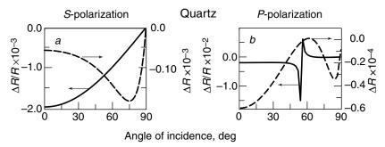
**Figure 2.10.** Reflectivity  $\Delta R/R$  (solid line) and absorption depth  $\Delta R$  (dashed line) of 1-nm layer ( $n_2=1.3, k_2=0.1$ ) on quartz ( $n_3=1.412$ ) for (a) s-polarized and (b) p-polarized radiation versus angle of incidence  $\varphi_1$  at  $n_1=1$ ,  $\nu=3000$  cm<sup>-1</sup>.
