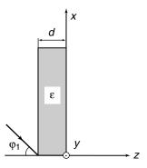
Figure 3.8. Coordinate system and optical constants in Vinogradov model.
