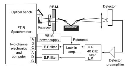
**Figure 4.52.** Schematic of optical potential-modulation (PM)-IRRAS setup and of two-channel electronic processing. PEM = photoelastic modulator, BP = bandpass, LP = low-pass, HP = high-pass. Reprinted, by permission, from D. Blaudez, T. Buffereau, J. C. Cornut, B. Desbat, N. Escares, M. Pezolet, and J. M. Turlet, *Appl. Spectrosc.* **47**, 869 (1993), p. 871, Fig. 2. Copyright © 1993 Society for Applied Spectroscopy.
