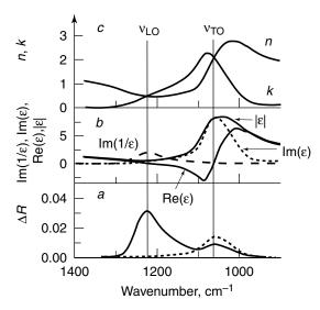
**Figure 3.11.** (a) Calculated ATR spectra of SiO<sub>2</sub> layer 2.5 nm thick on Ge for s-polarization (short-dashed line) and p-polarization (solid line) at  $\varphi_1 = 15^\circ$ ; (b) dispersion of TO (short-dashed line) and LO (long-dashed line) energy loss functions and  $|\varepsilon|$  and Re( $\varepsilon$ ) (solid line) of SiO<sub>2</sub>; (c) dispersion of refractive index n and extinction coefficient k of CVD SiO<sub>2</sub> after Rakov [52].
