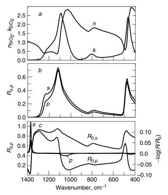
**Figure 2.14.** (a) Dispersion of optical constants n and k of fused quartz [75]; specular reflectance of quartz  $R_{0,s}$  and  $R_{0,p}$  obtained at (b)  $\varphi_1=20^\circ$  and (c)  $\varphi_1=80^\circ$ , plus s- and p-polarized IRRAS spectra of transparent layer with optical constants  $n_2=1.5$ ,  $k_2=0$ , and  $d_2=10$  nm on quartz surface.
