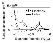
**Figure 3.45.** (a) Current-voltage curve of (100) Ge electrode in 1 *M* HClO<sub>4</sub> electrolyte taken when spectra shown in Fig. 3.44 were measured. Scan rate 10 mV ⋅ s<sup>-1</sup>. (b) Free-electron and free-hole absorption during potential scan under same conditions as in Fig. 3.43. Adapted, by permission, from F. Maroun, F. Ozanam, and J.-N. Chazalviel, *Surf. Sci.* **427-428**, 184 (1999), p. 185, Fig. 1 and p. 188, Fig. 3. Copyright ⊚ 1999 Elsevier Science B.V.
