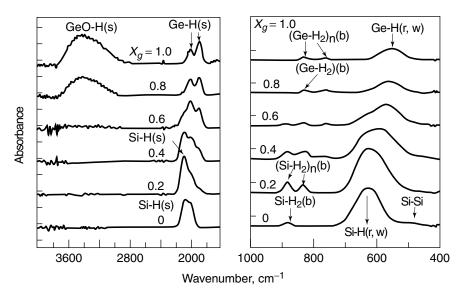
**Figure 5.19.** IR absorption of a-SiGe:H deposited at  $T_s = 200^{\circ}$ C for various values of  $X_g = \text{GeH}_4/(\text{GeH}_4 + \text{SiH}_4)$ . Reprinted, by permission, from Y.-P. Chou and S.-C. Lee, *J. Appl. Phys.* **83**, 4111 (1998). Copyright © 1998 American Institute of Physics.
