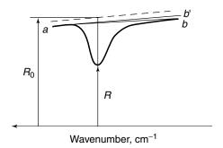
**Figure 3.71.** Scheme of drawing base line in IRRAS spectrum of film on metal surface: a-b', recommended baseline.
