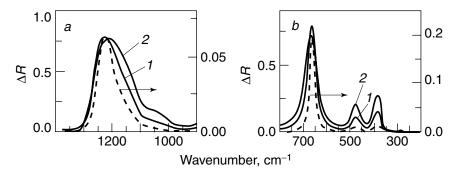
**Figure 3.16.** Simulated p-polarized IRRAS spectra of (a) SiO<sub>2</sub> films (1) 2 nm and (2) 4 nm thick located at Si\_Al interface (solid lines) and 2 nm thick at air Al interface (dashed line) at  $\varphi_1=80^\circ$  and (b)  $\alpha$ -Fe<sub>2</sub>O<sub>3</sub> films (1) 20 nm and (2) 40 nm thick at IKS-35–Fe interface (solid lines) and 20 nm at air Fe interface (dashed line) at  $\varphi_1=75^\circ$ .
