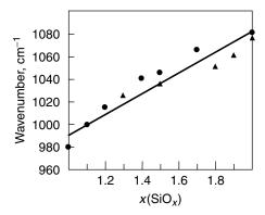
**Figure 5.4.** Band maximum of TO stretching mode of Si-O-Si bonds: symbols — experiment; solid line — calculation from Eq. (5.7). Reprinted, by permission, from H. Ono, T. Ikarashi, K. Ando, and T. Kitano, *J. Appl. Phys* **84**, 6064 (1998). Copyright © 1998 American Institute of Physics.
