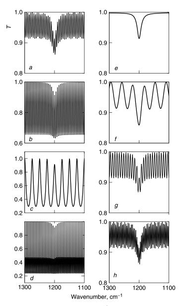
**Figure 2.5.** Dependence of normal-incidence  $(\varphi_1=0^\circ)$  transmission spectra of 100-nm layer, whose optical parameters are  $\varepsilon_\infty=2.3,\ \nu_0=1200\ {\rm cm}^{-1},\ \gamma=15\ {\rm cm}^{-1},\ S=0.015,$  on (a-d) refractive index and (e-h) thickness of substrate. Substrates are plane–parallel plates 3 mm thick with  $n_3$  values of (a) 1.35, (b) 2.0, (c) 3.4, and (d) 4.0 and with  $n_3=1.35$  and thicknesses  $d_3$  of (e) 0, (f) 0.1, (g) 0.5, and (h) 1 mm.
