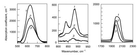
**Figure 5.16.** Typical IR absorption spectra of PECVD a-Si:H film obtained in pure silane at several substrate temperatures: (1) 50, (2) 100, and (3) 250°C. Reprinted, by permission, from K. Zellama, L. Chahed, P. Sladek, M. L. Theye, J. H. von Bardeleben, and P. Roca i Cabarrocas, *Phys. Rev. B* **53**, 3804 (1996). Copyright ⊚ 1996 American Physical Society.
