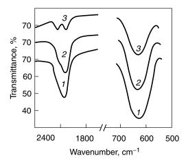
**Figure 5.17.** IR transmission spectra of a-Si:H film (1) before and (2) after 3 s and (3) 10 s annealing by CO<sub>2</sub> laser ( $\lambda = 10.6~\mu m,~p = 100~W \cdot cm^{-2}$ ). Reprinted, by permission, from H. Gleskova, V. V. Ilchenko, V. A. Skryshevsky, and V. I. Strikha, *Czech J. Phys.* **43**, 169 (1993). Copyright © 1993 Czech Journal of Physics.
