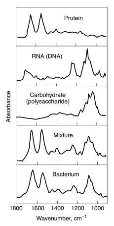
**Figure 7.56.** ATR FTIR spectra of bulk samples of (from top to bottom): protein (bovine serum albumin); RNA (ribonucleic acid, sodium salt yeast); carbohydrate, [p(+)-cellobiose]; mixture of appropriate proportions of protein, RNA, and carbohydrate found in bacterium, *Pseudomonas aeruginosa*. Reprinted, by permission, from P. A. Suci, J. D. Vrany, and M. W. Mittelman, *Biomaterials* **19**, 327 (1998), p. 330, Fig. 1. Copyright © 1998 Elsevier Science Ltd.
