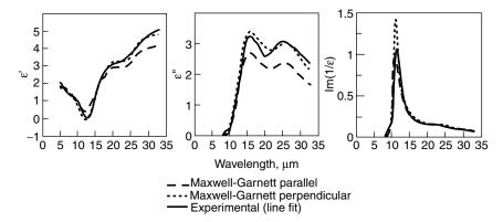
**Figure 3.60.** The TO and LO energy loss functions and real part of effective dielectric function, obtained using Maxwell-Garnett effective medium theory, are compared with corresponding experimental functions. Filling factor is 0.3 and pores are regarded as cylinders perpendicular to surface. Reprinted, by permission, from E. Wackelgard, *J. Phys. Condens. Matter* **8**, 4289 (1996), p. 4297, Fig. 4. Copyright © 1996 IOP Publishing Ltd.
