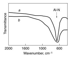
**Figure 5.31.** IR transmission spectra of AIN films deposited by CVD on Si substrate at (a) 67 Pa and 390°C and (b) 2.7 Pa and 340°C. Reprinted, by permission, from W. Zhang, Y. Someno, M. Sasaki, and T. Hirai, *Jpn. J. Appl. Phys.* **32**, L116 (1993). Copyright © 1993 Publication Board of Japanese Journal of Applied Physics.
