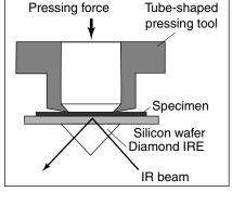
**Figure 4.16.** ATR configurations with diamond IRE. Film substrate is pressed against IRE: (a) pressing deforming layer; (b) pressing not deforming layer. Adapted, by permission, from G. Muller and C. Riedel, *Fres. J. Anal. Chem.* **365**, 43 (1999), pp. 43 (Fig. 1) and 44 (Fig. 2).
