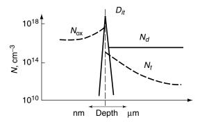
**Figure 6.20.** Diagram of spatial distribution of electron states in interfacial region. Here,  $D_{it}$  is density of surface state,  $N_t$ ,  $N_{ox}$ , and  $N_d$  are concentrations of bulk traps, oxide traps, and dopant, respectively.
