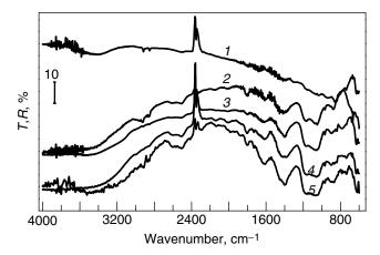
**Figure 2.51.** Comparison of IR spectra of oxidized surface compounds on galena (PbS) powder 50–70 μm size: (1) transmission of powder layer deposited from acetone on KBr plate after evaporation of acetone; (2) DTIFTS of powder layer deposited from acetone on ZnSe wedge (Section 4.2.2); (3) DRIFTS; (4) DRIFTS of 1:3 mixture with KBr; (5) transmission of 1:3 mixture of galena and KBr squeezed between two KBr windows.
