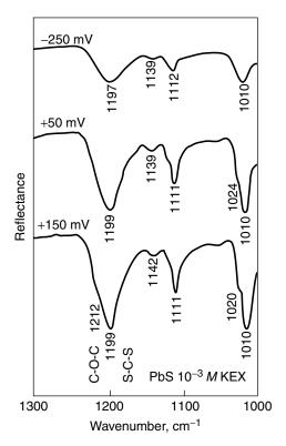
**Figure 7.38.** FTIR spectra of KEX adsorbed on galena at different potentials in 0.05~M Na<sub>2</sub>B<sub>4</sub>O<sub>7</sub> (pH 9.2) and  $10^{-3}$  KEX solution. Reprinted, by permission, from J. O. Leppinen, C. I. Basilio, and R. H. Yoon, *Int. J. Miner. Process.* **26**, 259 (1989), p. 269, Fig. 10. Copyright © 1989 Elsevier Science Publishers B.V.
