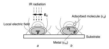
**Figure 3.62.** Polarization of metal particle in incident electric field. Thin lines represent electric field produced by induced dipole  $\mathbf{p}$  in particle. Metal particle is modeled by prolate ellipsoid. Adsorbed molecule is modeled by thin layer covering metal core.
