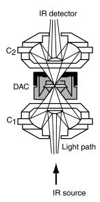
**Figure 4.34.** Schematic diagram of on-axis Cassegrain optics with diamond anvil cell (DAC) for IR transmission microspectroscopy; C<sub>1</sub> and C<sub>2</sub> are Cassegrain mirrors. Reprinted, by permission, from J. C. Chervin, B. Canny, J. M. Besson, and Ph. Pruzan, *Rev. Sci. Instrum.* **66**, 2595–2598 (1995), p. 2596, Fig. 1. Copyright © American Institute of Physics.
