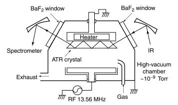
**Figure 4.43.** Scheme of ATR system for monitoring surface reactions in PECVD reactor. Reprinted, by permission, from Y. Miyoshi, Y. Yoshida, S. Miaziki and M. Hirose, *J. Non-Crystalline Solids* 198–200, 1029 (1996), p. 1030, Fig. 1. Copyright © 1996 Elsevier Science B.V.
