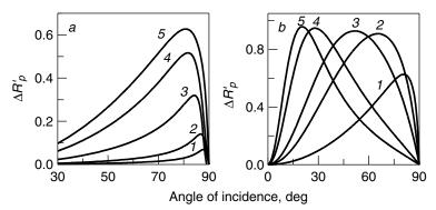
**Figure 2.30.** Angular dependence of band intensity  $\Delta R_p'$  in IRRAS of SiO<sub>2</sub> layer at immersion medium–Al interface;  $n_2 = 0.568$ ,  $k_2 = 0.356$  [2],  $n_3 = 18.55$ ,  $k_3 = 56.26$  [75], v = 1230 cm<sup>-1</sup> (vLO); (a)  $n_1$ : (1) 1, (2) 1.46, (3) 2.4, (4) 3.4, (5) 4.0,  $d_2 = 1$  nm; (b)  $n_1 = 4.0$ ,  $d_2$ : (1) 1, (2) 5 (3), 10, (4) 40, and (5) 80 nm.
