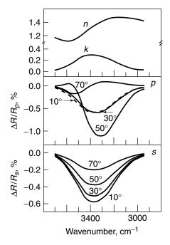
**Figure 3.20.** Simulated s- and p-polarized IRRAS spectra and optical constants  $k_2$  and  $n_2$  of 1-nm thick water layer on quartz as function of angle of incidence.
