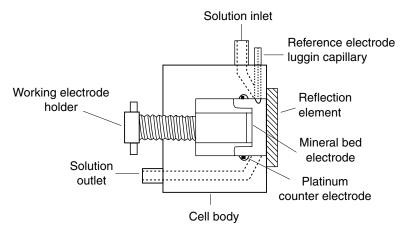
**Figure 4.51.** SEC-MIR cell constructed for in situ FTIR studies of reactions on mineral-particle bed electrodes. Reprinted, by permission, from J. O. Leppinen, C. I. Basilio, and R. H. Yoon, *Int. J. Min. Process.* **26**, 259 (1989), p. 260, Fig. 1. Copyright © 1989 Elsevier Science Publishers B.V.
