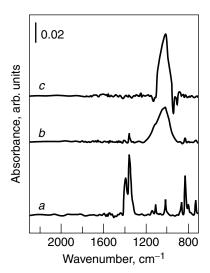
**Figure 2.48.** DRIFT spectra of *p*-nitrobenzoic acid adsorbed on Ag powders with particle sizes of (a) 2, (b) 5, and (c) 11  $\mu$ m. Reprinted, by permission, from H. S. Han, C. H. Kim, and K. Kim, *Appl. Spectrosc.* **52**, 1047 (1998), p. 1051, Fig. 5. Copyright © 1998 Society for Applied Spectroscopy.
