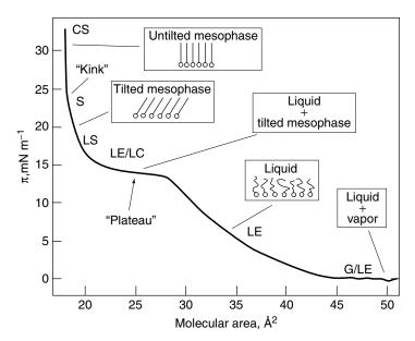
**Figure 3.79.** Surface pressure  $(\pi)$  versus molecular area isotherm of pentadecanoic (C<sub>15</sub>) acid L monolayer on pure water at about 30°C. Various features of isotherm can be identified with different structural phases. Adapted, by permission, from D. K. Schwartz, *Surf. Sci. Reports* **27**, 241 (1997), p. 248, Fig. 1. Copyright © 1997 Elsevier Science B.V.
