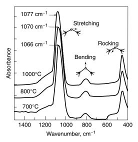
**Figure 5.1.** IR absorption spectra of  $SiO_2$  layer grown by annealing Si in dry oxygen at temperatures 700, 800, and  $1000^{\circ}$ C. Reprinted, by permission, from G. Lucovsky, M. J. Manitini, J. K. Srivastava, and E. A. Irene, *J. Vac. Sci. Technol. B* **5**, 530 (1987). Copyright © 1987 American Vacuum Society.
