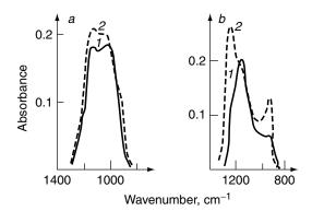
**Figure 6.14.** IRRAS spectra in p-polarized radiation at 75° of (a) thermal and (b) chemical oxides: (1) unannealed; (2) after thermal annealing at 300°C for 1 h.
