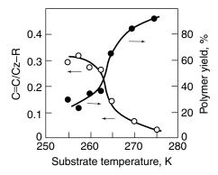
**Figure 7.50.** Values of C=C/Cz-R (○) and polymer yield (●) of NVCz film deposited by vapor deposition polymerization at various substrate temperatures. Reprinted, by permission, from M. Tamada, H. Koshikawa, and H. Omichi, *Thin Solid Films* **292**, 164 (1997), p. 167, Fig. 7. Copyright © 1997 Elsevier Science S.A.
