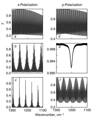
**Figure 2.6.** The *s*- and *p*-polarized oblique-incidence transmission spectra of 100-nm layer with optical parameters listed in Fig. 2.5. Layer is located on surface of 0.5-mm plane–parallel Si plate ( $n_3 = 3.4$ ). Spectra are obtained at  $\varphi_1$  values of (a, d) 40°, (b, e) 74°, and (c, f) 85°.
