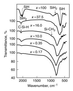
**Figure 5.20.** IR absorption spectra of a-SiC:H as function of silane fraction  $X = \text{SiH}_4/(\text{SiH}_4 + \text{CH}_4) \times 100\%$  in gas mixture. Reprinted, by permission, from A. S. Kumbhar, D. M. Bhusari, and S. T. Kshirsagar, *Appl. Phys. Lett.* **66**, 1741 (1995). Copyright © 1995 American Institute of Physics.
