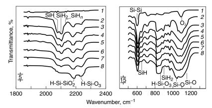
**Figure 5.24.** IR normal-incidence transmission spectra of (1) Si-substrate and (2-8) PS samples upon UV illumination for various times: (2) 0, (3) 10, (4) 20, (5) 30, (6) 40, (7) 60, and (8) 100 min.
