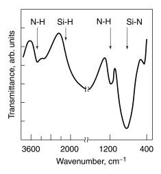
**Figure 5.12.** IR transmission spectrum of thin silicon nitride film produced by CVD of SiH<sub>4</sub> + N<sub>2</sub> at 65 $^{\circ}$ C. Reprinted, by permission, from T. Inukai and K. Ono, *Jpn. J. Appl. Phys.* **33**, 2593 (1994). Copyright © 1994 Publication Board of Japanese Journal of Applied Physics.
