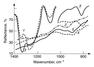
**Figure 6.9.** IRRAS ( $\varphi=75^{\circ}$ ) of Al–PSG–Si structures after thermal annealing at  $T \geq 450^{\circ}$ C for 1 h (curves labeled as in Fig. 6.8).
