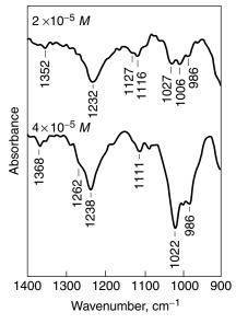
**Figure 7.27.** ATR spectra of pyrite particles after conditioning at two different concentrations of potassium ethyl xanthate (KEX). Reprinted, by permission, from J. O. Leppinen, *Int. J. Miner. Process.* **30**, 245 (1990), p. 251, Fig. 4. Copyright © 1990 Elsevier Publishers B.V.
