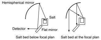
**Figure 4.31.** Scheme of how energy is maintained nearly constant with different salt bed height in cup in technique shown in Fig. 4.30. Reprinted, by permission, from F. Fondeur and B. S. Mitchell, *Spectrochim. Acta A* **56**, 467 (2000), p. 469, Fig. 3. Copyright © 2000 Elsevier
