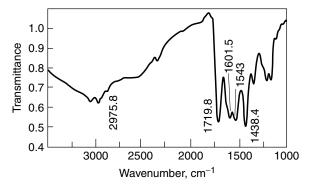
**Figure 7.52.** FTIR spectrum of maleic anhydride deposited on iron plate. Reprinted, by permission, from S. Bistac, M. F. Vallat, and J. Schultz, *Appl. Spectrosc.* **51**, 1823 (1997), p. 1824, Fig. 3. Copyright © 1997 Society for Applied Spectroscopy.
