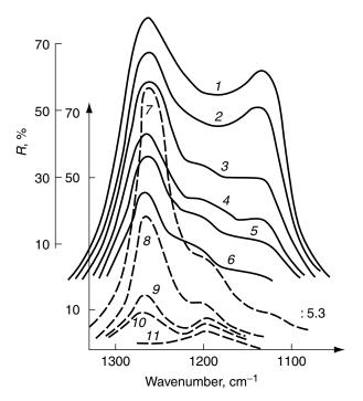
**Figure 5.33.** IRRAS spectra of  $SiO_2 - (n^+)Si$  structures at oxide thicknesses d of (1) 400, (2) 348, (3) 307, (4) 223, (5) 192, (6) 138, (7) 76, (8) 38, (9) 9, (10) 6, and (11) 2.5 nm.
