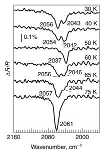
**Figure 7.5.** Spectra showing results of heating Pt(110) surface that has been exposed to 0.12 L of CO at 30 K. Heating to 50 K leads to disappearance of low-frequency band, and further heating to 65 K results in reappearance of higher frequency band. Reprinted, by permission, from R. K. Sharma, W. A. Brown, and D. A. King, *Chem. Phys. Let.*, **291**, 1−6 (1998), p. 3, Fig. 3. Copyright ⊚ 1998 Elsevier Science B.V.
