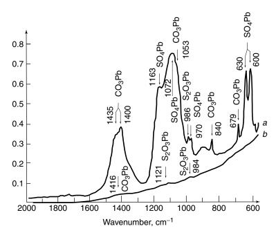
**Figure 7.16.** DRIFTS of two 5- $\mu$ m galena samples prepared by dry grinding. Samples (a) and (b) are p- and n-type semiconductors, respectively. Reprinted, by permission, from J. M. Cases and P. de Donato, *Int. J. Mineral Process.* **33**, 49 (1991), p. 54, Fig. 2. Copyright © 1991 Elsevier Science B.V.
