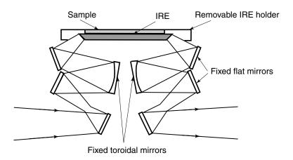
Figure 4.12. Optical scheme of horizontal ATR (HATR) accessory.
