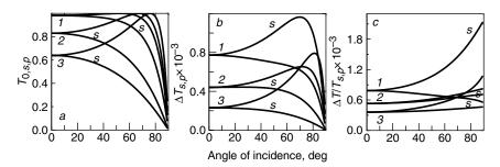
**Figure 2.2.** (a) Dependence of s- and p-polarized transmittance  $T_{0,s,p}$  of bare substrates, (b) absorption depth  $\Delta T_{s,p}$ , and (c) transmissivity  $\Delta T/T_{s,p}$  on angle of incidence:  $n_1=1$ ,  $d_2=1$  nm,  $n_2=1.564$ ,  $k_2=0.384$ ,  $\nu=1200$  cm<sup>-1</sup>; (1)  $n_3=1.35$  (CaF<sub>2</sub>), (2) 2.4 (ZnSe), (3) 4.0 (Ge).
