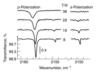
**Figure 7.12.** Transmission spectra of 0.6 ML of CO adsorbed at NaCl(100). Angle of incidence is 45°. Reprinted, by permission, from J. Heidberg, E. Kampshoff, R. Kuhnemuth, M. Suhren, and H. Weiss, *Surf. Sci.* **269/270**, 128 (1992), p. 131, Fig. 2. Copyright © 1999 Elsevier Science B.V.
