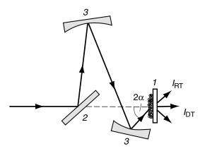
**Figure 4.22.** Optical scheme of diffuse-transmission accessory with side illumination of powder sample: (1) sample; (2, 3) directing and focusing mirrors, respectively. Reprinted, by permission, from V. P. Tolstoy, *Methods of UV-Vis and IR Spectroscopy of Nanolayers*, St. Petersburg University Press, St. Petersburg, 1998, p. 155, Fig. 4.25. Copyright © 1998 St. Petersburg University Press.
