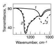
**Figure 6.11.** The *p*-polarized spectra from IRRAS (at  $\varphi = 75^{\circ}$ ) of (1) Si wafer, (2) Al–SiO<sub>2</sub>–Si, and (3) SiO<sub>2</sub>–Si.
