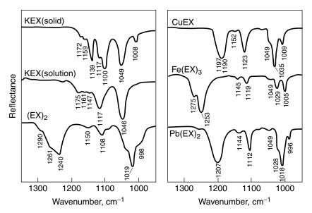
**Figure 7.23.** ATR spectra of reference compounds of ethyl xanthate. Reprinted, by permission, from J. O. Leppinen, C. I. Basilio, and R. H. Yoon, *Int. J. Miner. Process.* **26**, 259 (1989), p. 262, Figs. 2 and 3. Copyright ⊚ 1989 Elsevier Publishers B.V.
