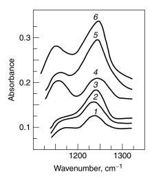
**Figure 6.4.** The *p*-polarized spectra from IRRAS of silicon oxide on Si at 75° incidence (1–3) before and (4–6) after In<sub>2</sub>S<sub>3</sub> deposition. Thickness of silicon oxide, *d*: (1) 1.0, (4) 2.5, (2) 2.0, (5) 4.5 (3), 4.0, and (6) 6.0 nm. Reprinted, by permission, from S. S. Kilchitskaya, T. S. Kilchitskaya, V. A. Skryshevsky, V. I. Strikha, and V. P. Tolstoy. *Zhurnal prikladnoi spektroskopii* **48**, 445 (1988). Copyright ⊚ 1988 Publishing House "Nauka i technika."
