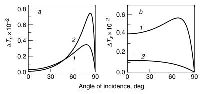
**Figure 2.3.** Angular dependence of absorption depth (a)  $\Delta T_p$  at  $\nu_{\text{LO}} = 1220 \text{ cm}^{-1}$  ( $n_2 = 0.54$ ,  $k_2 = 0.44$ ) and (b)  $\Delta T_s$  at  $\nu_{\text{TO}} = 1075 \text{ cm}^{-1}$  ( $n_2 = 2.15$ ,  $k_2 = 1.66$ ) for SiO<sub>2</sub> layer 1 nm thick on two substrates: (1)  $n_3 = 1.35$  and (2)  $n_3 = 4.0$ ;  $n_1 = 1$ . Optical constants of SiO<sub>2</sub> layer correspond to those of layer obtained by chemical deposition [2].
