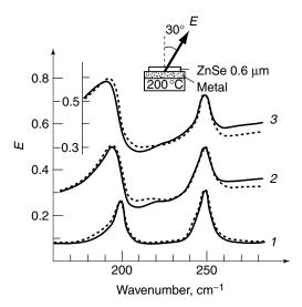
**Figure 3.10.** The p-polarized thermostimulated radiation spectra of 0.6- $\mu$ m ZnSe film on (1) Al, (2) Cr, and (3) Ti. Points are experimental data; solid curves are calculated. Reprinted, by permission, from E. A. Vinogradov, *Phys. Rep.* **217**, 159 (1992), p. 200, Fig. 25. Copyright © 1992 Elsevier.
