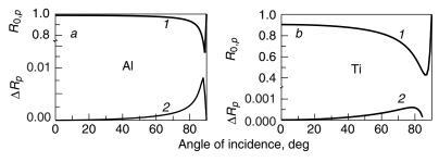
**Figure 2.7.** Dependence on angle of incidence of (1) reflectance  $R_{0,p}$  of bare substrate and (2) absorption depth  $\Delta R_p$  for 1-nm layer  $(\hat{n}_3 = 1.564 - 0.384\hat{i})$  at (a) Al  $(\hat{n}_3 = 18.6 - 77\hat{i})$  and (b) Ti  $(\hat{n}_3 = 6.5 - 14.8\hat{i})$  substrate;  $\nu = 1200$  cm<sup>-1</sup>; p-polarization, one reflection.
