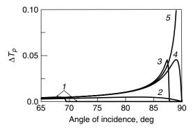
**Figure 2.25.** Dependence on angle of incidence of absorption depth  $\Delta T_p$  at  $\nu=1200~{\rm cm}^{-1}$  in p-polarized transmission spectrum of 1-nm film of model organic substance ( $n_2=1.564$ ,  $k_2=0.384$ ) located at interface of two media with refractive indices  $n_1$  and  $n_3$ : (1) 2.372 and 2.22, (2) 2.22 and 2.372, (3) 2.374 and 2.372, (4) 2.372 and 2.374, (5)  $n_1=n_3=2.372$ .
