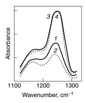
**Figure 6.2.** IR absorption spectra for Ti–SiO<sub>X</sub>–p-Si solar cells with oxide layer thicknesses of (1, 2) 2.5 nm and (3, 4) 5.0 nm (1, 3) before and (2, 4) after UV irradiation for 200 h. Reprinted, by permission, from S. S.Kilchitskaya, T. S.Kilchitskaya, G. D.Popova, and V. A.Skryshevsky, *Thin Solid Films* **346**, 226 (1999). Copyright ©1999 Elsevier Science.
