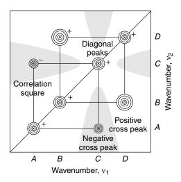
**Figure 3.51.** Schematic contour map of synchronous 2DIR correlation spectrum. Shaded areas represent negative-intensity regions. Adapted, by permission, from I. Noda, A. E. Dowrey, and C. Marcott, *Appl. Spectrosc.* **47**, 1317 (1993), p. 1318, Fig. 2. Copyright © 1993 Society for Applied Spectroscopy.
