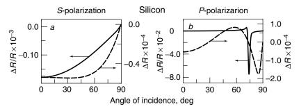
**Figure 2.9.** Reflectivity  $\Delta R/R$  (solid line) and absorption depth  $\Delta R$  (dashed line) of 1-nm layer ( $n_2=1.3, k_2=0.1$ ) on Si ( $n_3=3.433$ ) for (a) s-polarized and (b) p-polarized radiation versus angle of incidence  $\varphi_1$  at  $n_1=1, \nu=3000$  cm<sup>-1</sup>.
