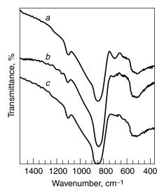
**Figure 5.28.** IR transmittance spectra of laser deposited  $GeO_X$  thin films on Si substrate at three substrate temperatures: (a) ambient, (b)  $100^{\circ}C$ , and (c)  $300^{\circ}C$ . Reprinted, by permission, from S. Witanachchi and P. J. Wolf, *J. Appl. Phys.* **76**, 2185 (1994). Copyright © 1994 American Institute of Physics.
