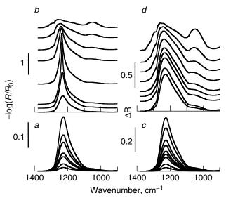
**Figure 3.12.** Simulated *p*-polarized IRRAS spectra of SiO<sub>2</sub> layers on Al as function of layer thickness,  $\varphi_1 = 80^\circ$ . Spectra are represented in (a,b) absorbance and (c,d) absorption depth  $\Delta R$  units. Layer thickness increases from lower to upper curve in series: (a) 1, 2, 4, 5, 8, 10, and 15 nm; (b) 50, 90, 110, 130, 160, 200, 300, and 500 nm; (c) 1, 2, 4, 5, 6, 8, 10, 15, and 20 nm; (d) 50, 90, 100, 110, 130, 160, 200, 300, and 500 nm.
