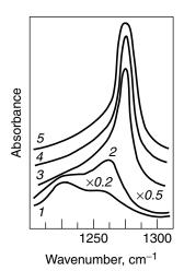
**Figure 6.6.** The *p*-polarized IRRAS at 75° incidence of AI $_{\rm SIO_x}$ -Si devices containing CVD oxide grown with reactant concentrations in ratio  $M = N_{\rm O_2}/N_{\rm TEOS}$  of (1)  $\sim$ 0, (2) 0.3, (3) 0.8, (4) 1.6, and (5) 2.0.
