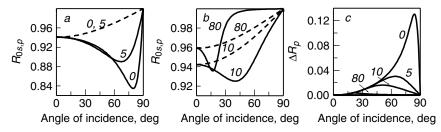
**Figure 2.38.** Dependence on angle of incidence of (a,b) p- (solid lines) and s- (dashed lines) polarized reflectance of Ge-air gap-Al MOATR configuration and (c) absorption depth of film on Ge for different air gaps; Ge:  $n_1 = 4.0$ ; film:  $\hat{n}_2 = 1.52 - 0.12i$ ,  $d_2 = 1$  nm; air gap:  $n_3 = 1.0$ ,  $k_3 = 0$ , values of  $d_3$  in nanometers are indicated on curves; Al:  $\hat{n}_4 = 1.94 - 22.10i$ ;  $v = 2800 \text{ nm}^{-1}$ .
