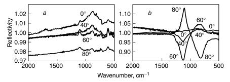
**Figure 3.17.** IRRAS spectra of  $SiN_x$  thin film on silicon wafer with (a) s-polarization and (b) p-polarization. Angles of incidence are shown. Silicon wafer without film is used as reference. Angle of incidence,  $\varphi_1 = 0^\circ$ , represents measurement at  $\varphi_1 = 11^\circ$  without any polarizer. Reprinted, by permission, from K. Yamamoto and H. Ishida, *Vibrational Spectrosc.* **8**, 1 (1994), p. 22, Fig. 21. Copyright © 1994 Elsevier Science B.V.
