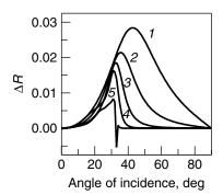
**Figure 2.40.** Angle-of-incidence dependence of absorption depth  $\Delta R$  at 2075 cm<sup>-1</sup> in *p*-polarized IRRAS spectra for 0.2-nm film with optical constants as for Fig. 2.39 in ZnSe–water layer–film–Pt system for water layer thicknesses: (1) 0.25, (2) 0.5, (3) 1, (4) 2, and (5) 5 μm.
