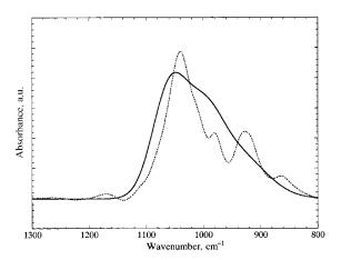
**Figure 7.10.** Spectra reconstructed from three component bands of sulfite (\_\_\_\_\_) and calculated from transmission spectrum of Chevreul's salt (.....). Reprinted, by permission, from J. Itoh, T. Sasaki, T. Ohtsuka, and M. Osawa, *J. Electroanal. Chem.* **473**, 256–264 (1999), p. 262, Fig. 8. Copyright © 1999 Elsevier Science S.A.
