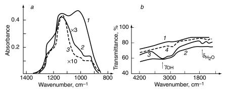
**Figure 6.13.** (a) IRRAS spectra in p-polarized radiation at 75° of InP oxides: (1) thermal, (2) chemical, and (3) anodic oxide. (b) IR transmission spectra of InP oxides: (1) thermal, (2) chemical, (3) anodic oxide, and (4) anodic oxide after thermal annealing at 300°C for 1 h.
