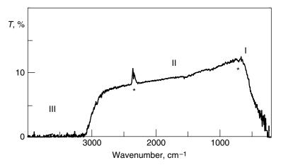
**Figure 1.3.** Absorption according to different mechanisms in transmission spectrum of a 2-mm-thick PbS plate. I – phonon absorption, II – transparency region, III – fundamental absorption. Asterisks indicate artifact due to atmosphere absorption.
