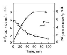
**Figure 5.25.** Absorption of PS layer in 1030–1170- and 2080–2140-cm<sup>-1</sup>spectral regions as function of duration of UV illumination.
