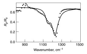
**Figure 3.2.** IRRAS spectra of MOS Si-photo-CVD SiO<sub>2</sub> 2 nm thick-Al system (CVD = Chemical vapor deposition): experiment (triangles) and two-oscillator simulation (solid line); p-polarization,  $\varphi_1 = 80^\circ$ . Reprinted, by permission, from R. Brendel, *Appl. Phys.* **A50**, 587 (1990), p. 591, Fig. 3a. Copyright © 1990 Springer-Verlag.
