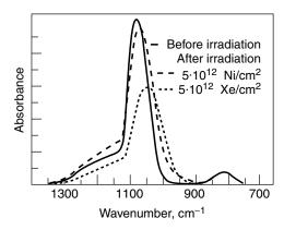
**Figure 6.23.** IR absorption of thermal  $SiO_2$  before and after irradiation by Xe and Ni at  $5 \times 10^{12}$  ions/cm<sup>2</sup>. Reprinted, by permission, from M. C. Busch, A. Slaoui, P. Siffert, E. Dooryhee, and M. Toulemonde, *J. Appl. Phys.* **71**, 2596 (1992). Copyright © 1992 American Institute of Physics.
