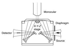
**Figure 4.36.** Optical configuration of reflectance FTIR microscope constructed on basis of Collector. Reprinted, by permission, from J. A. J. Jansen, J. H. Van Der Maas, and A. Posthuma De Boer, *Appl. Spectrosc.* **45**, 1149–1152 (1991), p. 1150, Fig. 1. Copyright © 1991 Society for Applied Spectroscopy.
