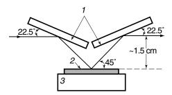
**Figure 4.10.** Scheme of single-reflection IRRAS accessory with horizontal sample: (1) directing mirrors; (2) sample; (3) sample holder. Reprinted, by permission, from J. Chatelet, H. H. Claasen, D. M. Gruen, I. Sheft, and R. B. Wright, *Appl. Spectrosc.* **29**, 185 (1975), p. 187, Fig. 1. Copyright © 1975 Society for Applied Spectroscopy.
