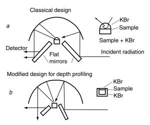
**Figure 4.30.** (a) Classical and (b) modified DRIFTS accessories for depth profiling of fibers. Reprinted, by permission, from F. Fondeur and B. S. Mitchell, *Spectrochim. Acta A* **56**, 467 (2000), p. 469, Fig. 2. Copyright © 2000 Elsevier Science B.V.
