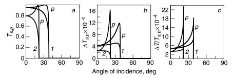
**Figure 2.24.** Dependence of s- and p-polarized (a) transmittance  $T_{s,p}$ , (b) absorption depth  $\Delta T_{s,p}$ , and (c) transmissivity  $\Delta T/T_{s,p}$  on angle of incidence of IR radiation: (1)  $n_1=2.4$ , (2)  $n_1=4.0$ ;  $n_2=1.564$ ,  $k_2=0.384$ ,  $\nu=1200$  cm<sup>-1</sup>,  $n_3=1.5$ .
