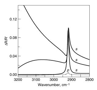
**Figure 2.22.** Reflectivity of film (S=0.004,  $\varepsilon_\infty=2.22$ ,  $\gamma=10~{\rm cm}^{-1}$ ,  $\nu=2920~{\rm cm}^{-1}$ ,  $d_2=2.5~{\rm nm}$ ) on BML substrate with buffer layer 750 nm thick characterized by  $n_3=1.4$  and  $k_3=0$  for p-polarization and, from bottom to top,  $k_3=0$ , 0.04, 0.08 for s-polarized radiation;  $n_1=1$ ,  $n_4=3.2$ ,  $k_4=23$ ,  $\varphi_1=85^\circ$ .
