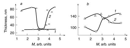
**Figure 5.15.** Thicknesses of (a)  $SiO_2$  and (b)  $Si_3N_4$  layers obtained from IR absorption spectra (1) before and (2) after annealing in wet oxygen at  $1050^{\circ}C$  during 5 h as functions of  $M=(4\%\ SiH_4+96\%\ Ar)/NH_3$ . Reprinted, by permission, from Yu. A. Averkin, N. K. Karmadonov, V. A. Skryshevsky, V. I. Strikha, and A. V. Kharlamov, *Ukrainian J. Phys.* **34**, 1817, (1989). Copyright © 1989 Institute of Theoretical Physics, National Academy of Science of Ukraine.
