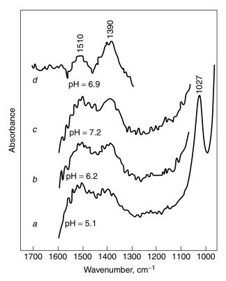
**Figure 7.15.** ATR-FTIR spectra of AI oxide with carbonate species adsorbed. Initial  $[NaHCO_3] = 0.001 \, M$  for spectra a, b, and c. Initial  $[NaHCO_3] = 0.010 \, M$  in  $D_2O$  for spectrum d. Band at 1027 cm<sup>-1</sup> in spectrum A is 0.019 a.u. Reprinted, by permission, from H. Wijnja and C. P. Schulthess, *Spectrochim. Acta A* **55**, 861 (1999), p. 866, Fig. 3. Copyright © 1999 Elsevier Science B.V.
