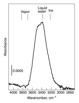
**Figure 7.13.** Infrared absorption of water adsorbed to NaCl(100) at  $-27^{\circ}$ C and 0.2 mbar of water. Coverage is calculated to be 1.5 ML. Reprinted, by permission, from M. Foster and G. E. Ewing, *Surf. Sci.* **427/428**, 102 (1999), p. 102, Fig. 1. Copyright © 1999 Elsevier Science B.V.
