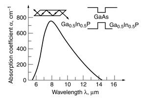
**Figure 6.19.** Intersubband absorption spectrum recorded at room temperature. Insets show  $45^{\circ}$  multipass waveguide configuration and band of tuning of lattice-matched  $GaAs-Ga_{0.5}In_{0.5}P$  heterostructure. Reprinted, by permission, from S. D. Gunapala, B. F. Levine, R. A. Logan, T. Tanbun-Ek, and D. A. Humphrey, *Appl. Phys. Lett.* **57**, 1802 (1990). Copyright © 1990 American Institute of Physics.
