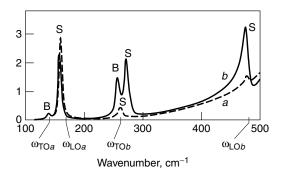
**Figure 3.56.** Calculated extinction cross section of CdTe sphere of radius 3  $\mu$ m with CdO coating of (a) 10 nm and (b) 100 nm thick; S and B denote surface and bulk mode absorption peaks, respectively. Reprinted, by permission, from R. Ruppin, *Surf. Sci.* **51**, 140 (1975), p. 145, Fig. 3. Copyright © 1975 North-Holland Publishing Company.
