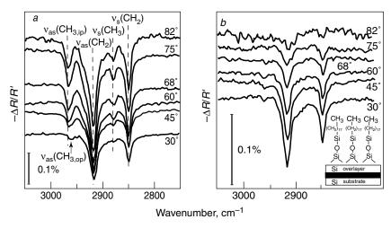
**Figure 2.20.** BML-IRRAS spectra of SAM of OTS on Si-CoSi<sub>2</sub>-Si substrate with 70-nm buffer layer as function of angle of incidence: (a) p-polarization, (b) s-polarization. Reprinted, by permission, from Y. Kobayashi and T. Ogino, *Appl. Surf. Sci.* **100/101**, 407 (1996), p. 409, Fig. 1. Copyright © 1996 Elsevier Science B.V.
