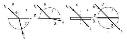
**Figure 2.1.** Optical schemes for recording oblique-incidence transmission spectra of nanolayers, in which layer is located (a, b) on surface of hemicylinder, (c) on surface of plane-parallel plate, (d) between two hemicylinders: (1) immersion medium with refractive index  $n_1$ , (2) layer under investigation of thickness  $d_2$  and with optical constants  $n_2$  and  $k_2$ , (3) transparent substrate with refractive index  $n_3$ .
