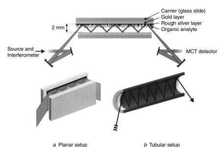
**Figure 4.9.** Setup for multiple IRRAS-SEIRA experiments showing (a) planar configuration and (b) tubular configuration. Analyte layer is deposited as thin film on top of silver film. Reprinted, by permission, from H. D. Wanzenböck, B. Mizaikoff, N. Weissenbacher, and R. Kellner, *Fresenius J. Anal. Chem.* **362**, 15 (1998), p. 17, Fig. 3. Copyright © 1998 Springer-Verlag.
