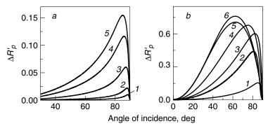
**Figure 2.28.** Angular dependence of band intensity  $\Delta R_p'$  in IRRAS of layers characterized by oscillator parameters  $\varepsilon_{\infty}=2.3,\ \gamma=15\ {\rm cm^{-1}},\ \nu_0=1200\ {\rm cm^{-1}},\ S=0.015$  and located at immersion medium–Al interface:  $n_3=19.52, k_3=57.7, \nu=1200\ {\rm cm^{-1}};\ (a)\ d_2=1\ {\rm nm},\ n_1:\ (1)\ 1,\ (2)\ 1.46,\ (3)\ 2.4,\ (4)\ 3.4,\ (5)\ 4.0;\ (b)\ n_1=4.0,\ d_2:\ (1)\ 1,\ (2)\ 5,\ (3)\ 10,\ (4)\ 20\ (5),\ 40\ {\rm and}\ (6)\ 80\ {\rm nm}.$
