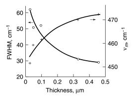
Figure 5.27. Frequency and the FWHM of ν<sub>LO</sub> band as functions of thickness of CaF<sub>2</sub> layer.
