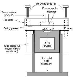
**Figure 4.32.** View of horizontal ATR accessory modified for measurements of IR spectra of powders. Reprinted, by permission, from C. M. Balik and W. H. Simendiger, *Polymer* **39**, 4723–4728 (1998), p. 4724, Fig. 1. Copyright © 1998 Elsevier Science Ltd.
