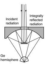
**Figure 4.37.** Configuration of typical ATR objective. Reprinted, by permission, from L. Lewis and A. J. Sommer, *Appl. Spectrosc.* **53**, 375–380 (1999), p. 376, Fig. 1. Copyright © 1999 Society for Applied Spectroscopy.
