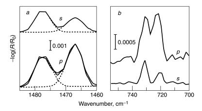
**Figure 3.81.** Split of methylene (a) scissors and (b) rocking mode in s- and p-polarized IRRAS of behenic acid ester L monolayer ( $\pi \approx 14~\text{mN} \cdot \text{m}^{-1}$ ) on pure (a) D<sub>2</sub>O and (b) H<sub>2</sub>O. Spectra were measured at 40° angle of incidence. Adapted, by permission, from C. R. Flach, A. Gericke, and R. Mendelsohn, *J. Phys. Chem. B* **101**, 58 (1997), pp. 61 (Fig. 6) and 64 (Fig. 12). Copyright © 1995 American Chemical Society.
