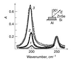
**Figure 3.9.** The *p*-polarized thermostimulated spectra of 0.6- $\mu$ m ZnSe film on buried metal layer (BML) substrates Si–Al with Si buffer layer thickness: (1) 0, (2) 2, and (3) 3  $\mu$ m. Points are experimental data; solid curves are calculated. Experimental points are shifted downward for spectra 1 and 2 by 0.06 and for spectrum 3 by 0.13 (reduction of background radiation).
