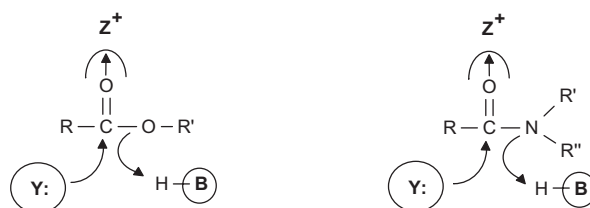
Fig. 3.2. Common catalytic groups of hydrolases involved in ester and amide bond hydrolysis ( Z^+ = electrophilic component polarizing the carbonyl group; Y: = nucleophilic group attacking the carbonyl C-atom; H-B = proton donor transforming the -OR' or -NR'R'' moiety into a better leaving group)
