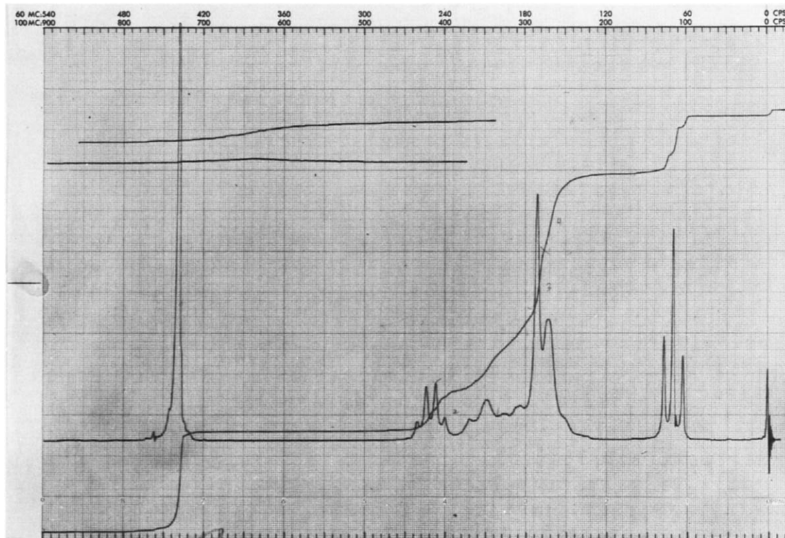
Fig. 2 NMR Spectrum of Meperidine Hydrochloride, U.S.P., Wyeth Lot No. F-665901. Solvent: deuterochloroform, internal standard: tetramethylsilane. Instrument: Jelco Model C-60 HL.
